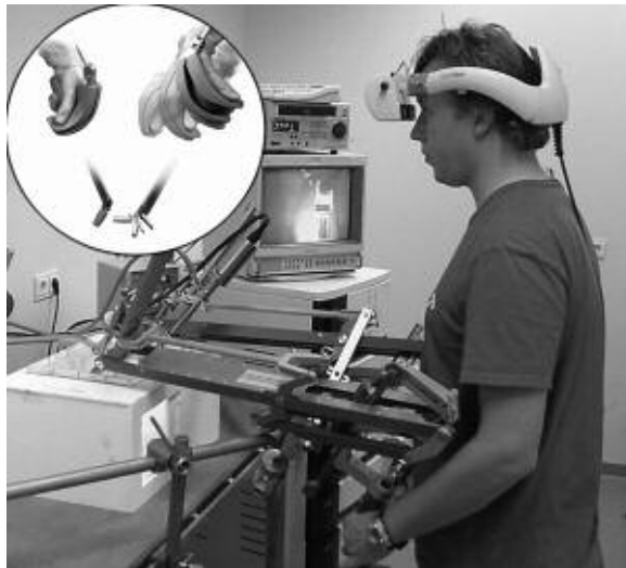
Figure 5.2. The Mechanical Manipulator in the experimental set-up. The picture shows two parallelogram mechanisms coupled to the table rail. The inset shows that movement directions of the handle correspond to identical movement directions of the instrument tip in all DOFs
