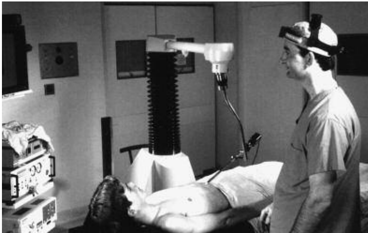
Figure 1.6. A “robotic” camera holder: the EndoAssist, controlled by head movements of the surgeon.
