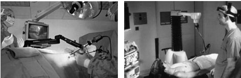
Figure 2.5. Motorised or “Robotic” camera holders: Left: AESOP (Computer Motion): a SCARA type electromechanical arm activated by voice control. Right: EndoSista (Armstrong Healthcare): a SCARA type electromechanical arm activated by head movements.
