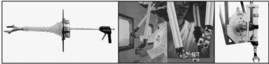
Figure 1.9. Three types of instruments used for handling nuclear material. Left: A relatively simple instrument with the gripper inside a bunker and the handle outside. Middle: Intuitive manipulation with a mechanical manipulator; The grippers inside the bunker (on the right) are mechanically connected with the operator's handles (on the left) outside, in 7DOFs. Right: An electro-mechanical arm (Slave). These arms can be manipulated from a remote location (Master), not shown here.
