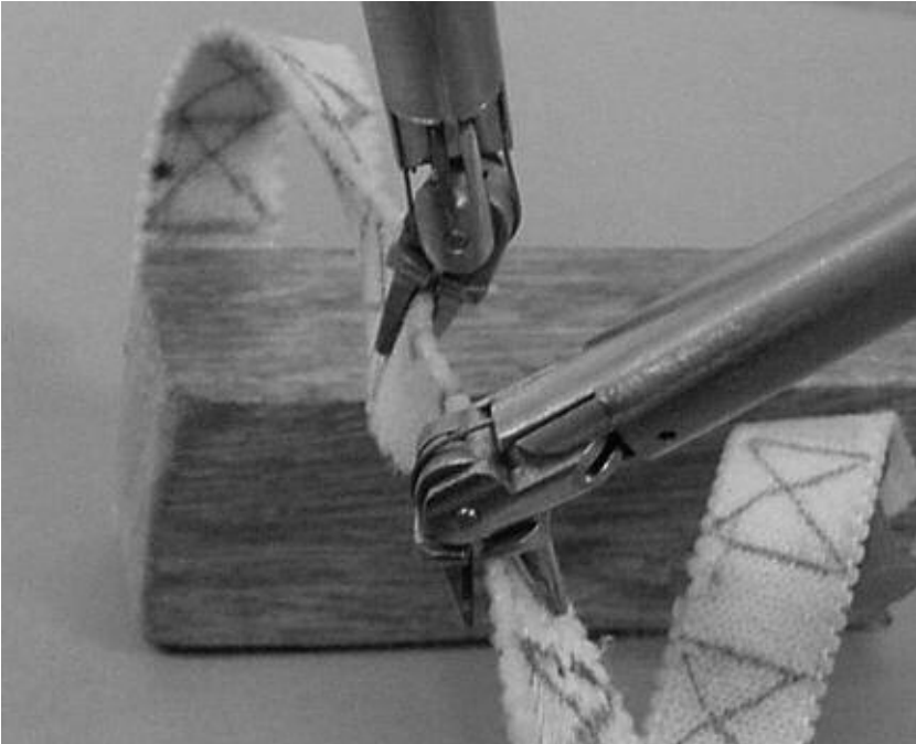
Figure 5.3. Experiment 2: rope-passing, manipulating a marked band with two instrument by grasping it at same side (MIM experiment)
