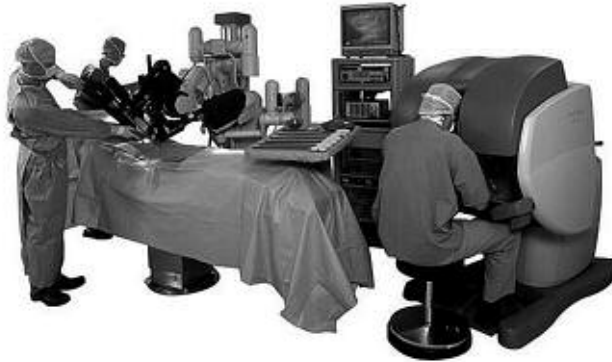
Figure 1.7. “Robotic” or Master-Slave telemanipulator (da Vinci®). On the left (behind the OR-table), the robotic arms (Slave) for controlling the endoscopic instruments and on the right the surgeon’s console (Master).
