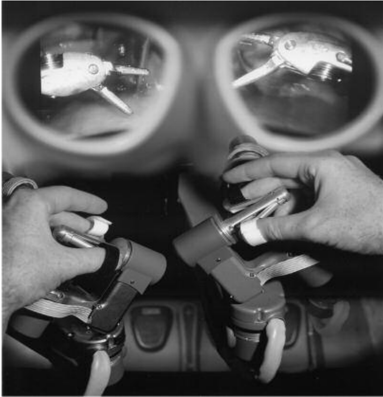
Figure 1.8. Intuitive control of the endoscopic instruments with 7 DOFs of the da Vinci® robot; the surgeon's handles are always in the same orientation as the instrument's tips, like with open surgery. (Picture by UMC-Utrecht)
