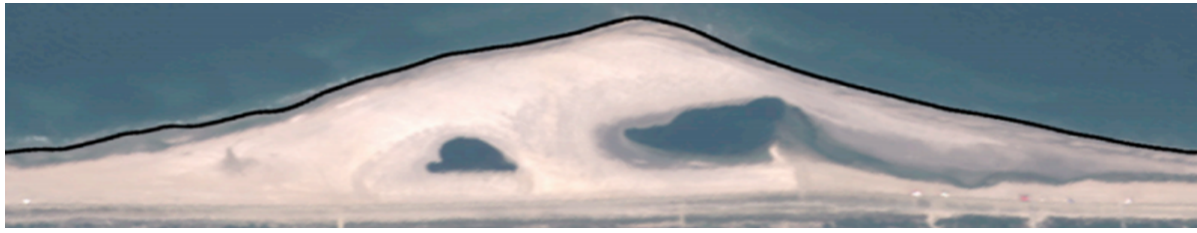
Figure 2.3: An example of the employment of the Satellite Derived Shorelines (SDS) detection algorithm for the Sand Engine study site. The resulting SDS is shown in black. (source: Hagenaars et al., 2018 )
