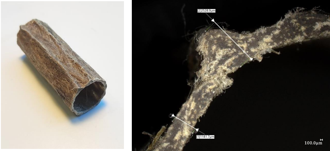
Figure 48: a. 'Ridges' formed by the pinching from the vacuum bag b. the ridge as seen under a microscope, showing the bundling of fibres
