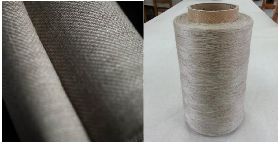
Figure 28 a : : Flaxdry BL360 , Source: eco-technilin.com , b: Lincore 520 flax roving, Source: www.circular-structures.com
