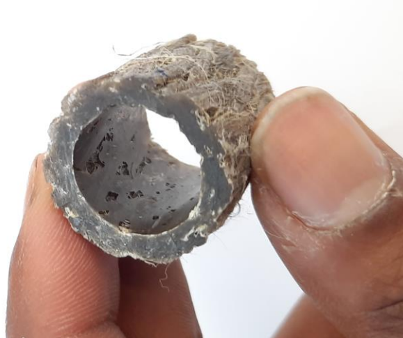
Figure 56: pre tensioned braided composite sample after diamond cutting. Defects within the cross section and a rougher surface finish to be noted
