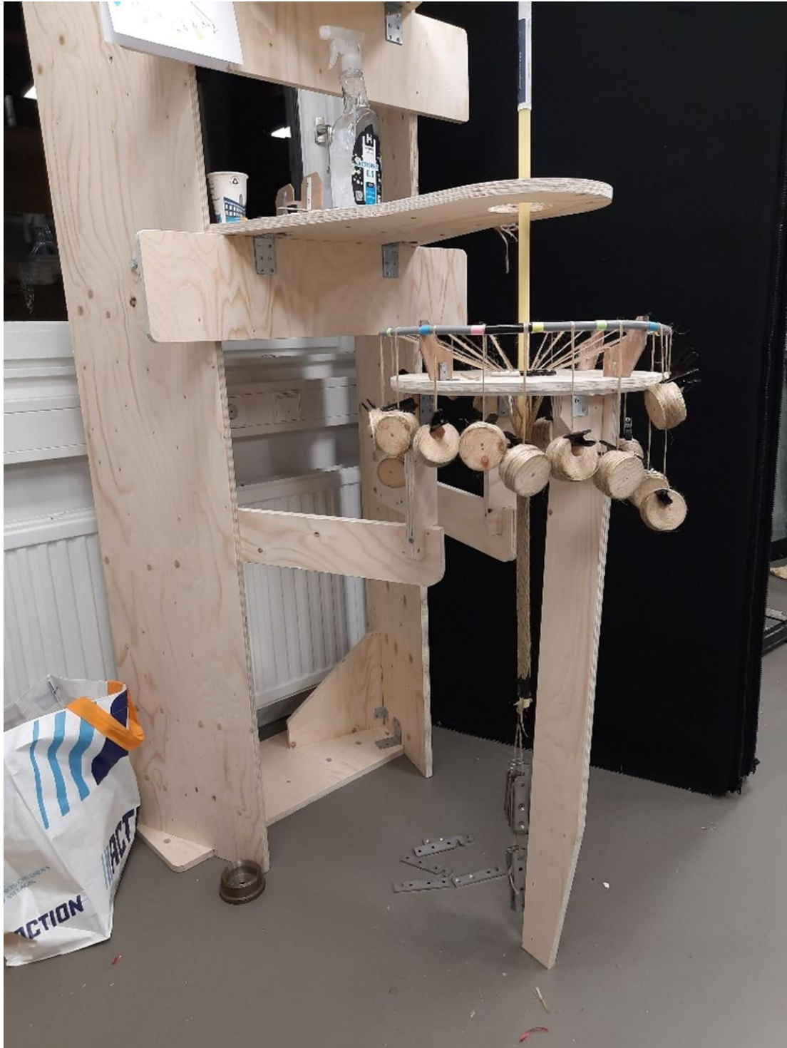
Figure 41: The final braiding apparatus, as built and used in the Think Room, Faculty of Architecture TU Delft.
