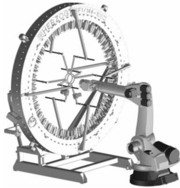
Figure 33: a. An example of a radial braid machine (courtesy Herzog USA), b. Photo of a 12 carrier braid machine at the Textielmuseum, Tilburg, NL
