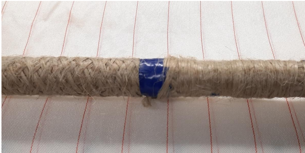
Figure 57: Series 5a and 5b prepared, with shallow braid reinforcement, and helical winding, respectively
