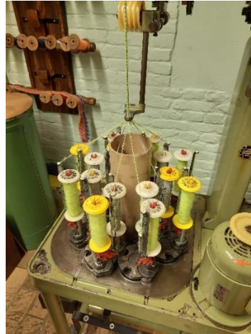
Figure 33: a. An example of a radial braid machine (courtesy Herzog USA), b. Photo of a 12 carrier braid machine at the Textielmuseum, Tilburg, NL
