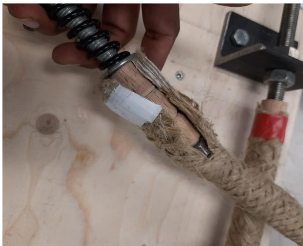
Figure 73: Sequence of joint fabrication- A montage/ 1. Required materials 2. Setup of the chord section on the jig, 3. Preparation of the clamping insert for the strut, 4. Insertion of the clamping block in the strut sleeve, 5. Tightening of the strut sock over the braid sleeve.
