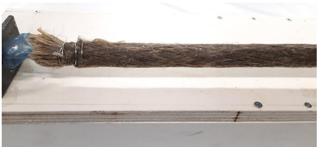
Figure 67: Pre tensioning applied to the resin soaked braided cordage, compacted against the discontinuous mandrel
