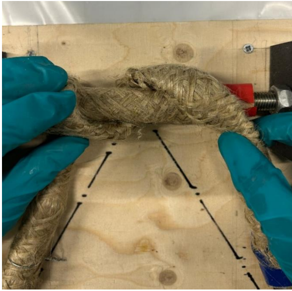
Figure 74: Sequence of joint preparation of the hollow strut 'sock' over the chord section.
