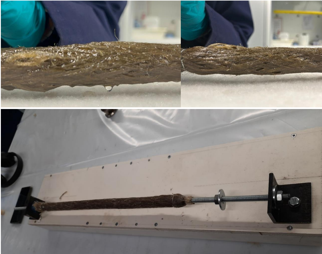
Figure 54: the pre tensioning rig for a single tubular sample, b. excess resin drip-off upon tensioning
