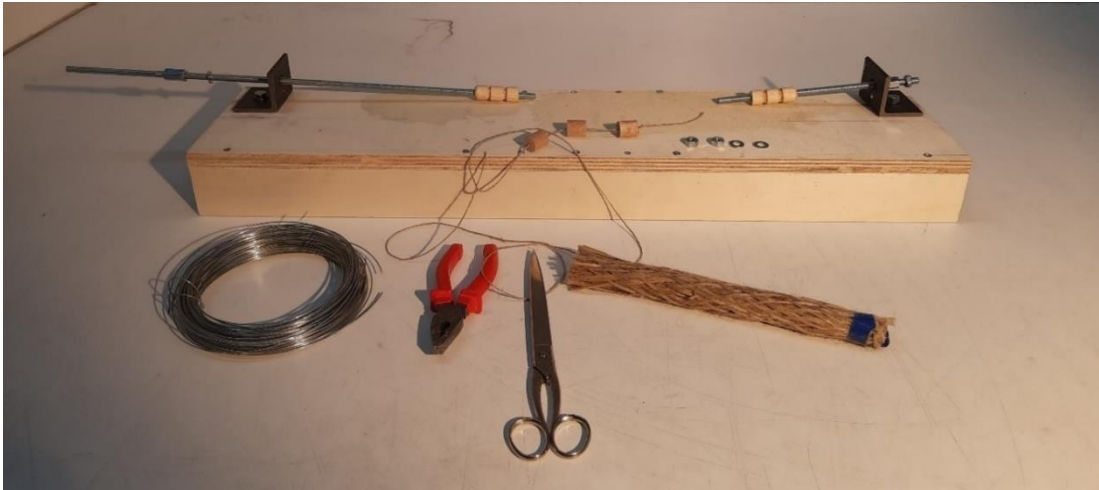
Figure 65: Setup to manufacture the strut compacted against the 'discontinuous mandrel'
