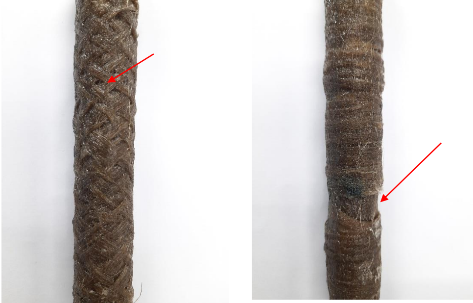
Figure 58: Series 5a and 5b after curing. 5a shows a visibly lower constriction between the shallow overbraid and the deep braids underneath. Series 5b shows similar effect with the helical winding, with a complete detachment of windings in some sections.
