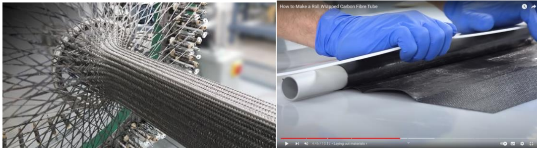
Figure 45: a. Braiding of carbon fiber, b. Roll wrapping carbon fiber prepregs to make a roll wrapped tube
