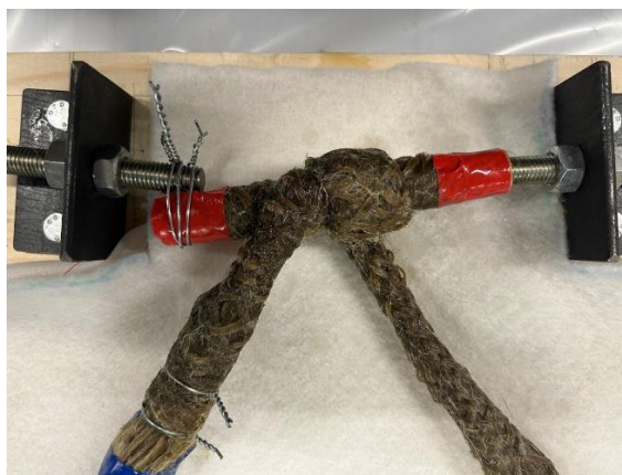
Figure 75: The joint section after resin application and pre-tensioning. The tension force fractures the timber in the chord section, compromising the joint geometry, but the tension is maintained. The final product is shown on the joint.
