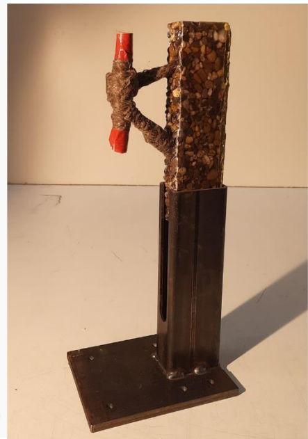
Figure 76: Proposal for joint testing. a. Sketch showing the fitting of the epoxy encased joint into the custom fabricated jig. b. Photographs of the specimen. The joint encasement did not fit inside the jig, and was later clamped to the front of the box section for the load test.
