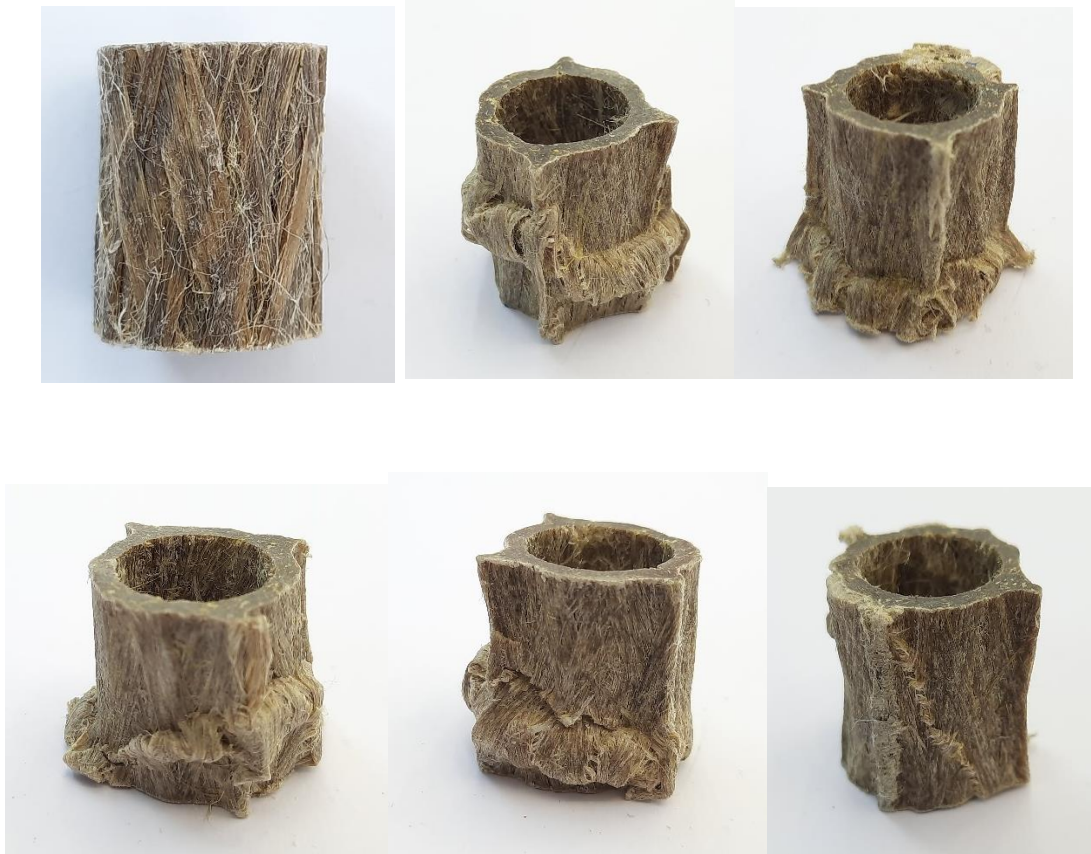
Figure 53: a. A sample of 6 layer braided composite before compressive test. b-f: compressive failure of 5 samples by microbuckling. F shows micro-buckling along the braid seam
