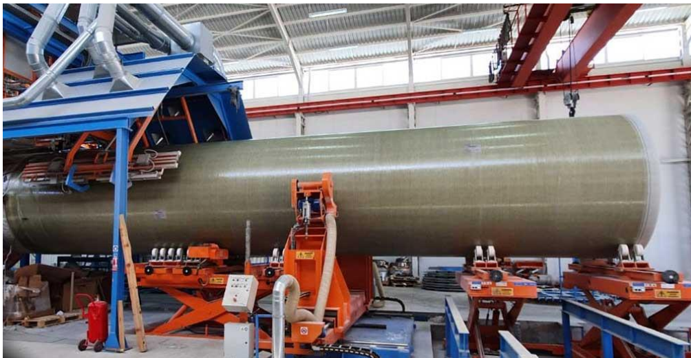
Figure 18: GRP pipe manufactured by filament winding. Source: (3 Incredible “Did You Know” Facts About GRP Pipes, 2020)
