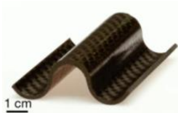
Figure 106: A corrugated carbon FRPC part fabricated by FROMP using vacuum-assisted resin-transfer moulding (Robertson, et al., 2018)
