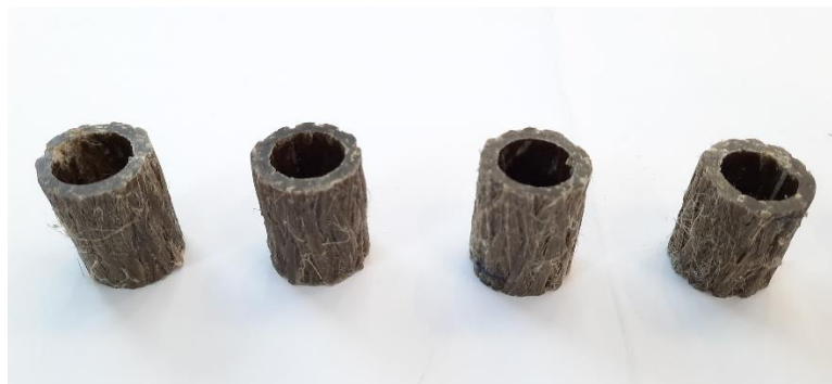
Figure 55: Cross section of pre tensioned braided composite showing defects
