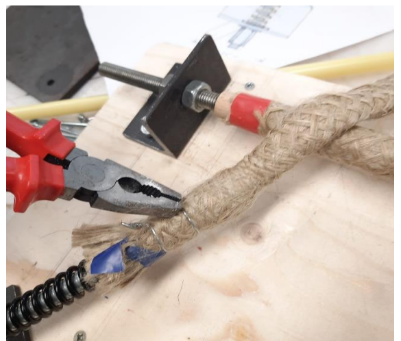
Figure 73: Sequence of joint fabrication- A montage/ 1. Required materials 2. Setup of the chord section on the jig, 3. Preparation of the clamping insert for the strut, 4. Insertion of the clamping block in the strut sleeve, 5. Tightening of the strut sock over the braid sleeve.
