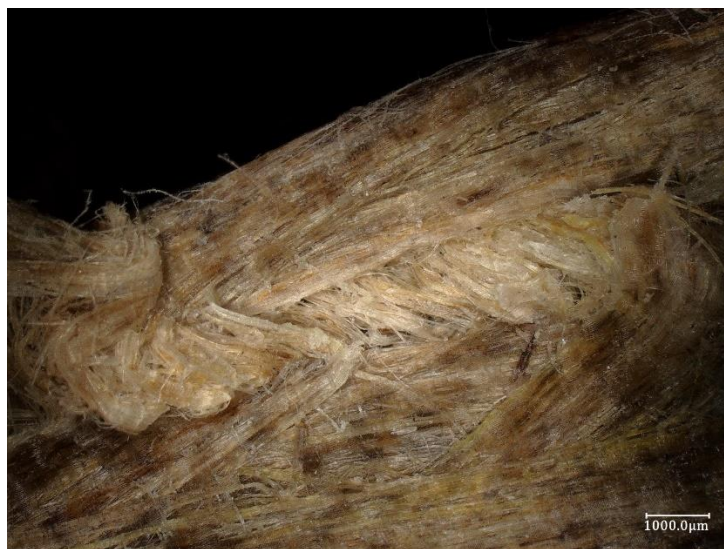
Figure 51: Fiber micro-buckling in the braided composite, as seen under a microscope
