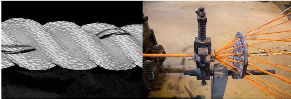
Figure 23: a. Twined rope structures (McKenna, Hearle, & O'Hear, 2004) b. The making of twisted rope, source: /www.ravenox.com
