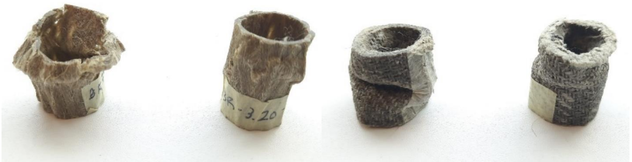
Figure 50: Failure pattern in braided composite (left) and woven composite (right)
