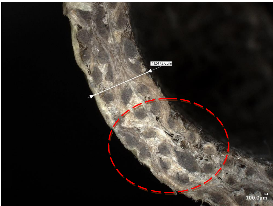
Figure 49: Cross section of woven flax composite as seen under microscope. The presence of voids and imperfections is apparent
