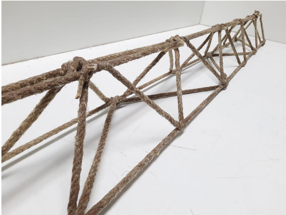
Figure 96: A prismoid portal frame constructed on the breadboard as a series of 3 tying cycles for each of the planes.
