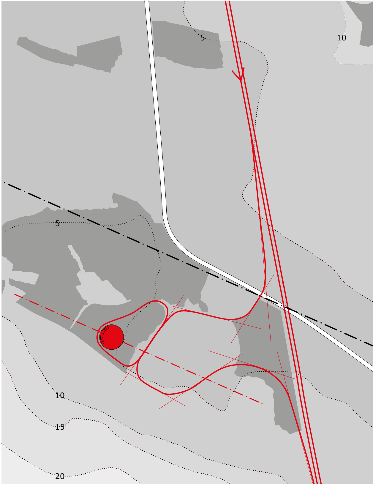
Figure 8 The Bois Brossard forms a roughly rectangular strip parallel to the axis of the Charente valley, covering the steep slope between plateau and valley, where to motorway makes the transition to the plateau. The road is an elongated loop, parallel to the slope to minimise the height difference, following the basic form of the forest.
