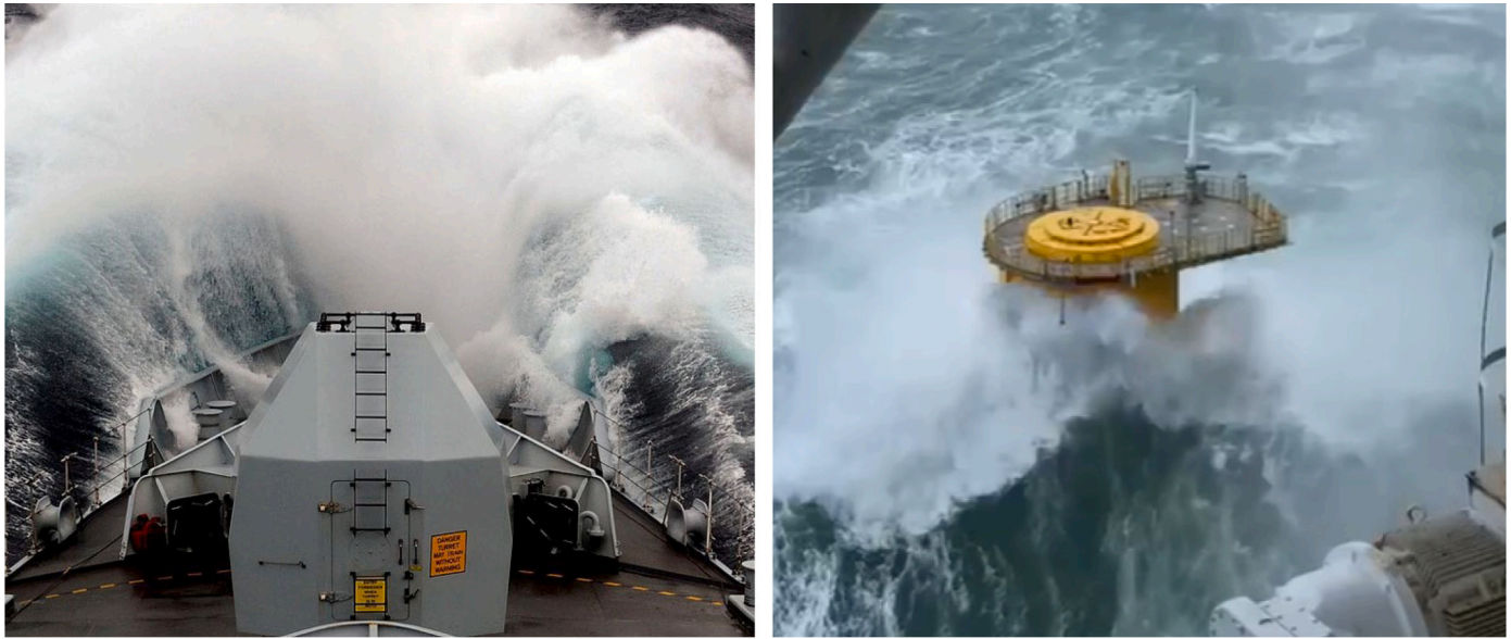
Fig. 1. Two examples of wave impacts on marine structures: a wave impacting HMS Edinburgh of the UK Royal Navy in 8 m waves on the South Atlantic (left; courtesy D. Rosenbaum, Royal Navy Media Archive [15], with permission) and a wave impacting a wind turbine foundation with a transition piece ~20 m above the calm water level close to Fécamp during storm Ciarán on 2 Nov. 2023 (right; courtesy K. King, with permission).
