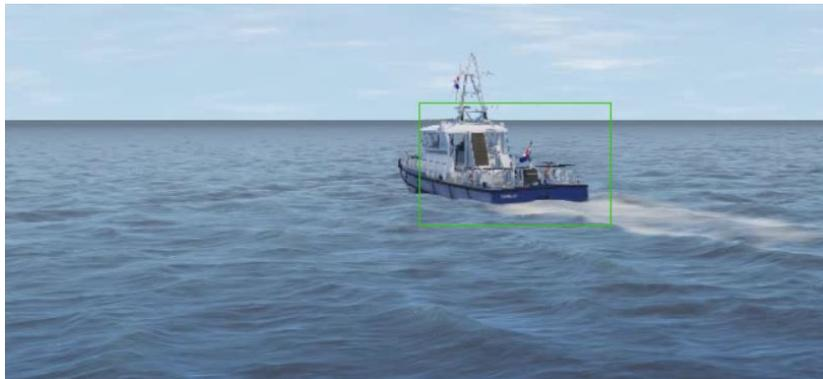
**Figure 3-13:** Wake of vessel causes small bearing offset
