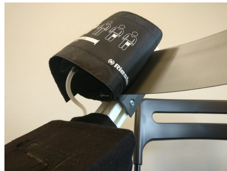
Figure 3.8: The cuff and preform in place
