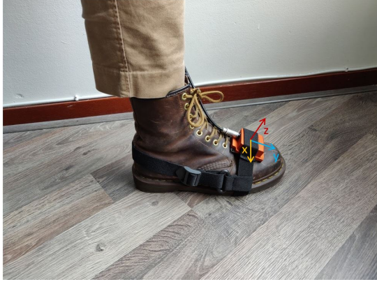
Fig. 2. Experimental setup with foot-mounted sensor.
