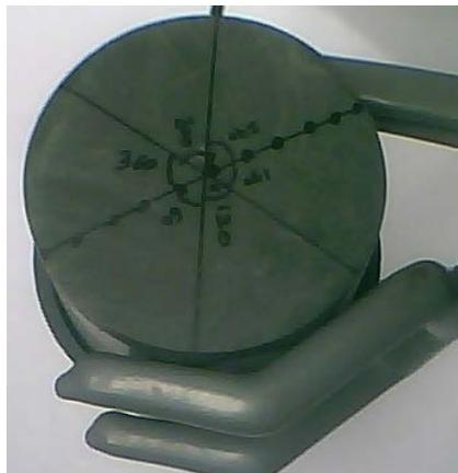
**Figure 3.24 DWM disdrometer to test the depth of edge effect**
