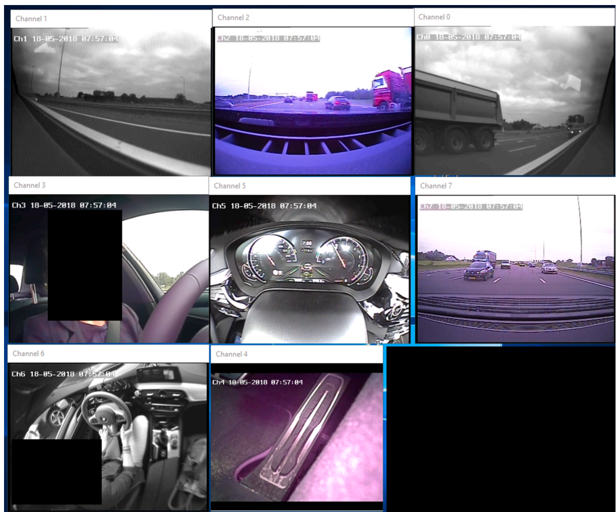
Fig. 1. Overview of the eight camera perspectives recorded by the TNO instrumentation in the time-synchronized visualisation by SWOV for each vehicle. In reading order: right mirror view, forward view, left mirror view, driver face, instrument panel, rear view, driver seat, pedal bay. The driver's face is occluded for privacy reasons.
