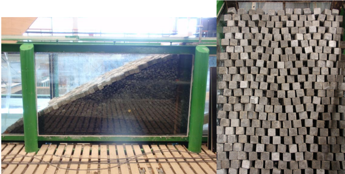
Figure 13. Top and side view model slope 1:2
