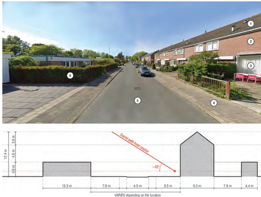
Figure 19: Street view at Rijsenhout and the approximate dimension of the housing and canyon size (source: Google Map)
