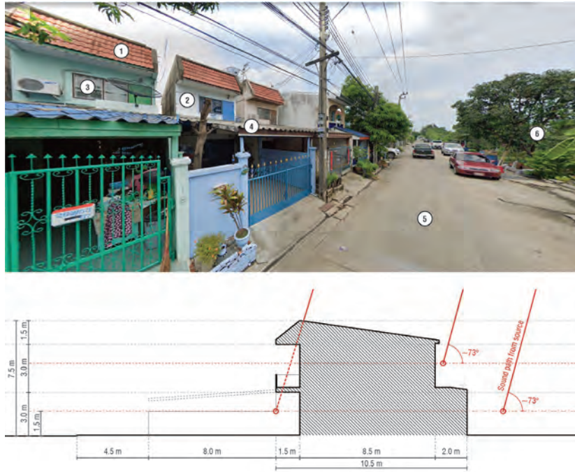
Figure 26: The existing condition of Chanlamat village and building typology with rough dimension (source: Google Map)
