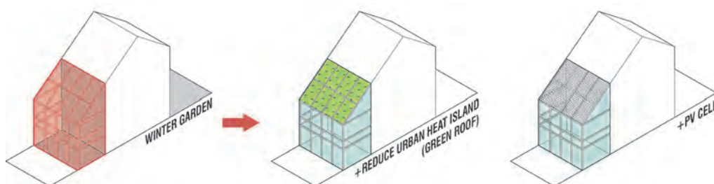
Figure 59: Winter garden proposal with different integral design solution for housing at Rijsenhout
