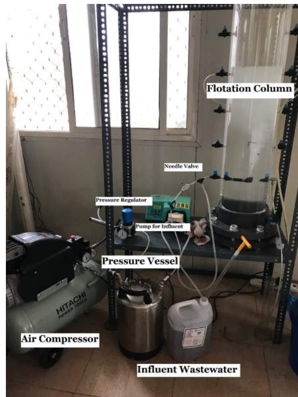
Figure 3.3: DAF set up at the LOTUS HR site in New Delhi
