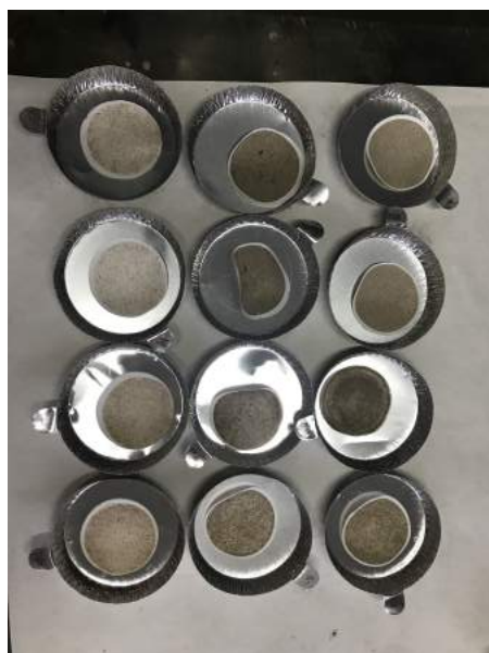
(a) Filters showing the TSS retained after oven drying (105 °C) for the Barapullah drain water.
