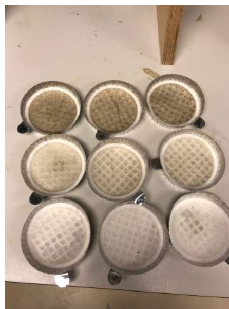
(b) Filters showing the TSS retained after oven drying (105 °C) for the canal water.
