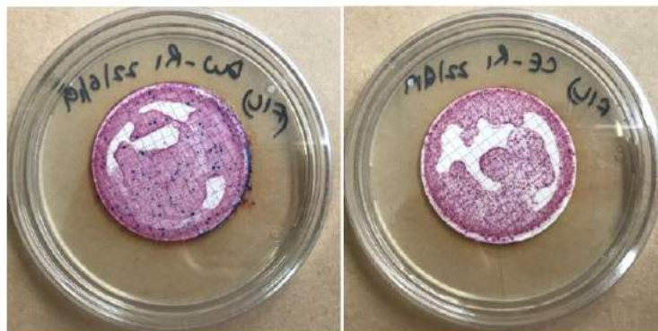
Figure 3.11: Plates for E-coli removal with membrane filtration from the drain water.
