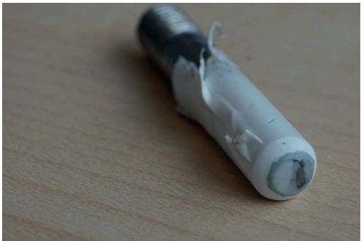
figure A.28: Tip of the thermode with PTFE cover (white) with little to no solder paste sticking to it.
