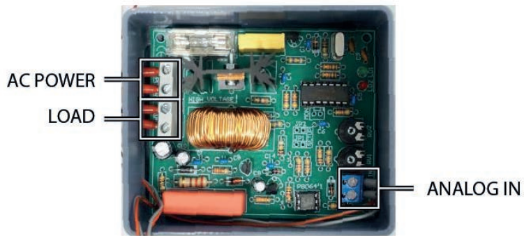
Figure 9: The AC dimmer module and its connections.
