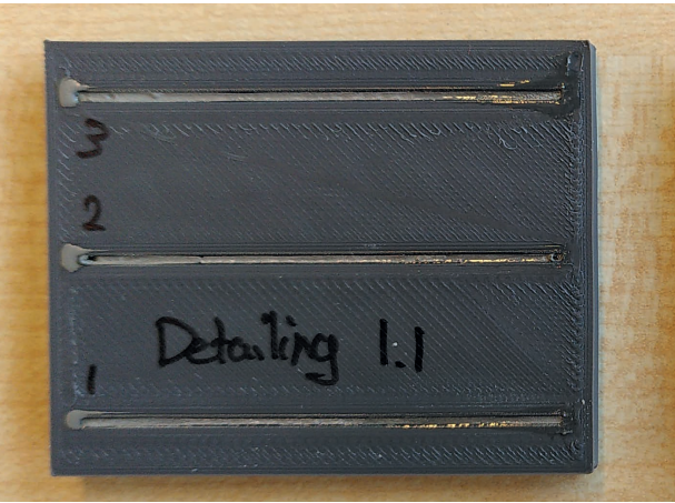
figure 6.4: The result of printing and curing solder paste using the example Gcode.
