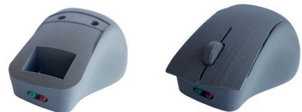
Figure 24: (left) The top cover printed separately and (right) placed onto the prototype.
