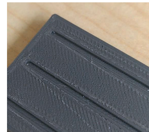
Figure 12: The channel recessed in the plastic part
