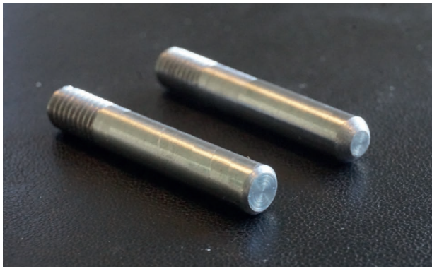
figure A.19: The two tips of the thermode.
