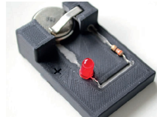
figure 3.1: The results of curing the solder paste in a convection oven from the previous master thesis research by M. Bon.
