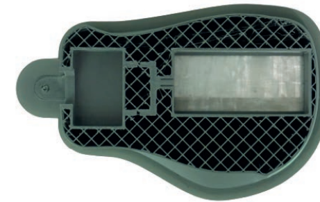
figure 7.1: The first part of the demonstrator printed with room for the battery holder.
