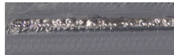
figure 3.9: Final results with uncured solder paste and solder balls.
