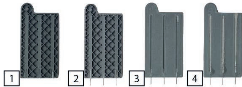
Figure 20: Four steps of printing over the lead of a component from left to right (1) print recessed channels for the lead to fit into. (2) insert leads into recessed channels (3) print recessed channel over the leads partly overlapping the lead and (4) print and cure solder paste in the channel creating a conductive interface between the lead and the solder paste trace.
