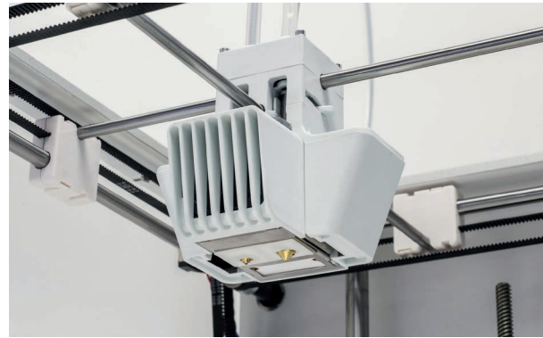
figure 4.3: The dual extrusion head of the Ultimaker 3
