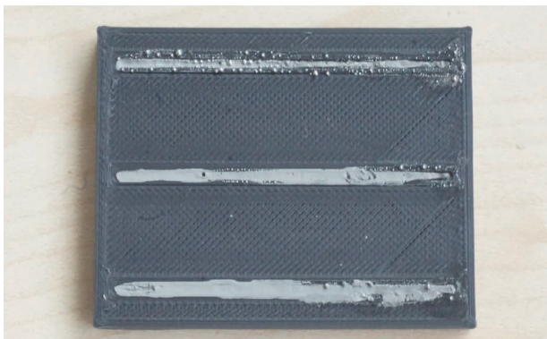
figure 3.13: Later test where the right temperature and air flow were used with good results.
