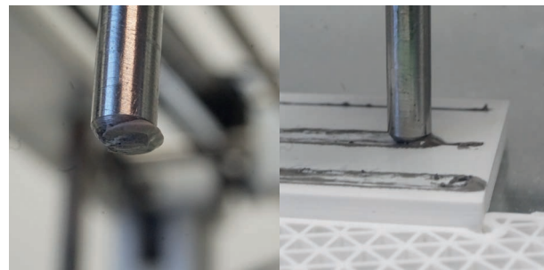
figure 3.4: Solder paste curing on the thermode rod and pushing the solder paste out of the channel.
