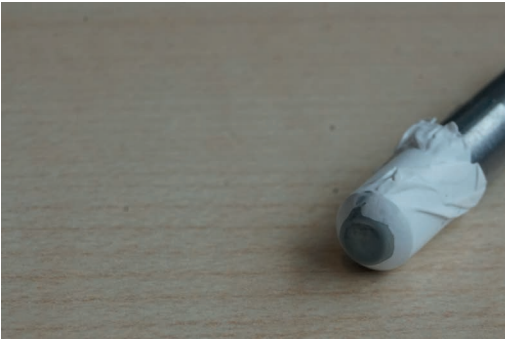
figure A.26: Tip of the thermode with PTFE cover (white) after printing
