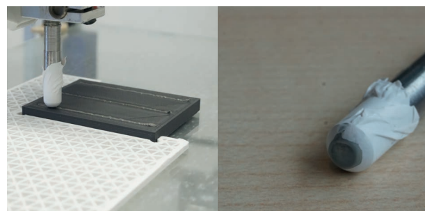
figure 3.5: The thermode rod with the PTFE tape, (left) and the tip of the thermode rod after curing (right).
