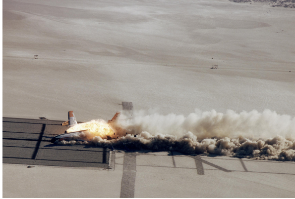
Figure 1.7: Full-scale crash test.
