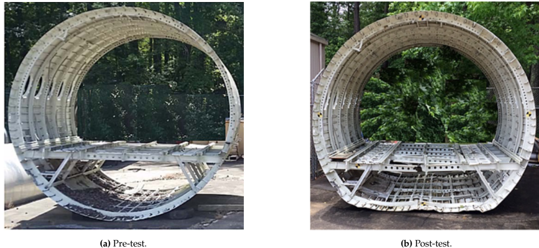
Figure 4.8: F-28 forward section without hat racks, seats, ATDs, and floor panels[58].
