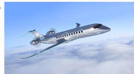
Figure 1.4: Embraer Energia H2 gas turbine E50-H2GT[7].
