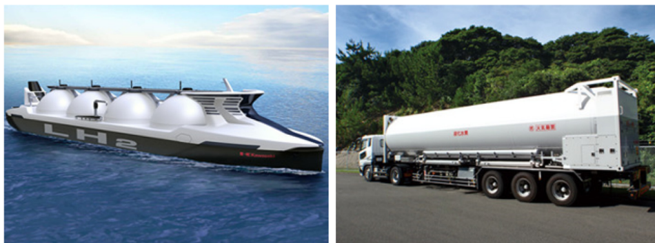
Figure 5.2: Left: Kawasaki heavy industry concept design for liquid hydrogen carriers and on the right: Cryogenic trailer [66].
