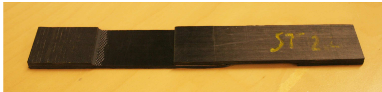
Figure 2.11: A lap shear test sample, with the tungsten layer positioned in between the carbon fiber composite coupons. Additional coupon material was added to the ends, in order to reduce force eccentricity.
