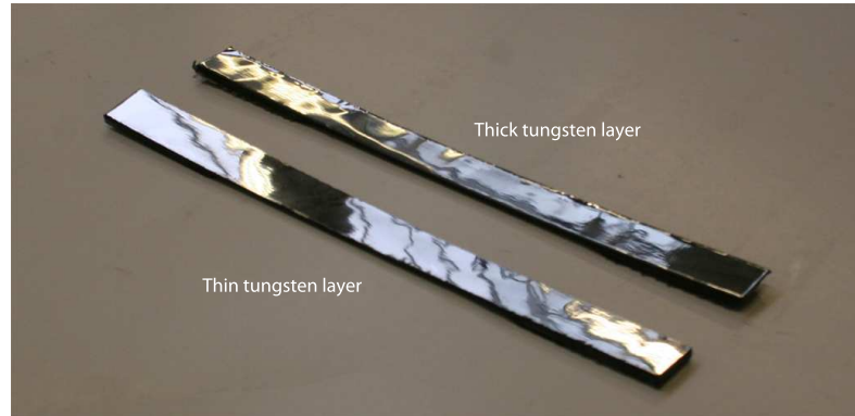
Figure 2.19: In-plane DLC-coated tungsten failure experienced during manufacturing in a tensile strength test sample.
