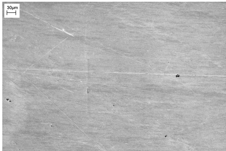
Figure 2.23: Secondary electron imaging of the unabraded tungsten foil, showing almost no impurities/inclusions. The lines/scratches were ascribed to handling errors. The scale bar indicates a distance of 30 \mu\text{m} .
