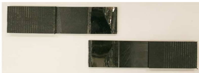
Figure 2.18: A special case of adherent failure was found for the DLC, where the tungsten adherent failed itself, over almost its entire surface.
