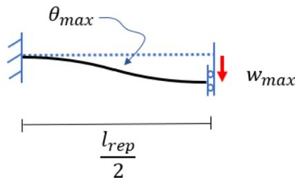
Figure 2.9: Schematic drawing of the floor deflection corresponding to the beam formula
