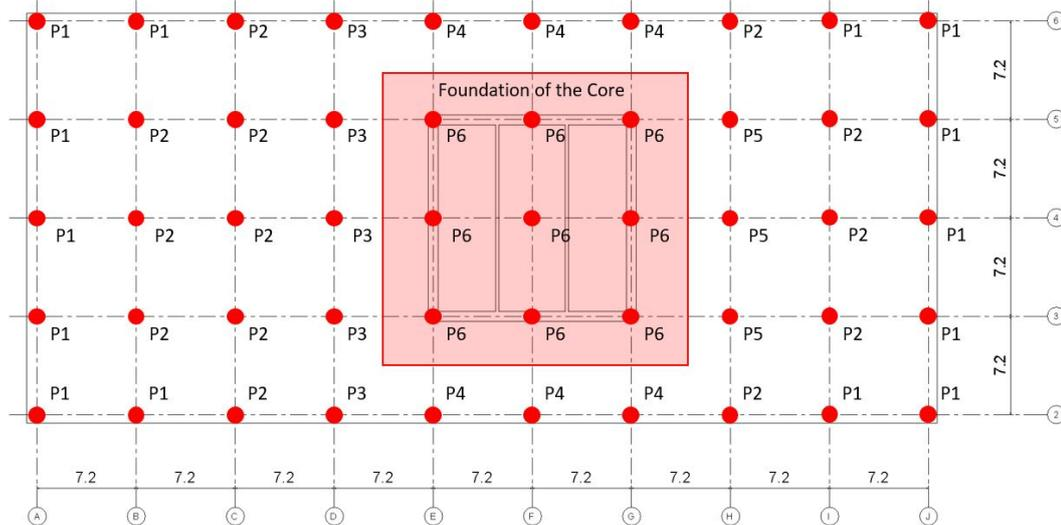
Figure 3.13: Locations of the supports with mentioning the groups used for the calculation
