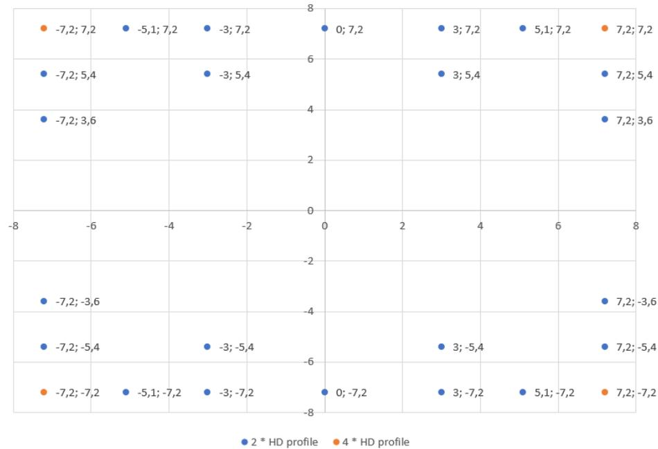
Figure A.10: The locations of the columns for the steel stability truss
