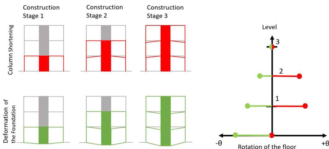
Figure 2.12: Schematic drawing of the rotation of the floors due to column shortening and displacements of the foundation
