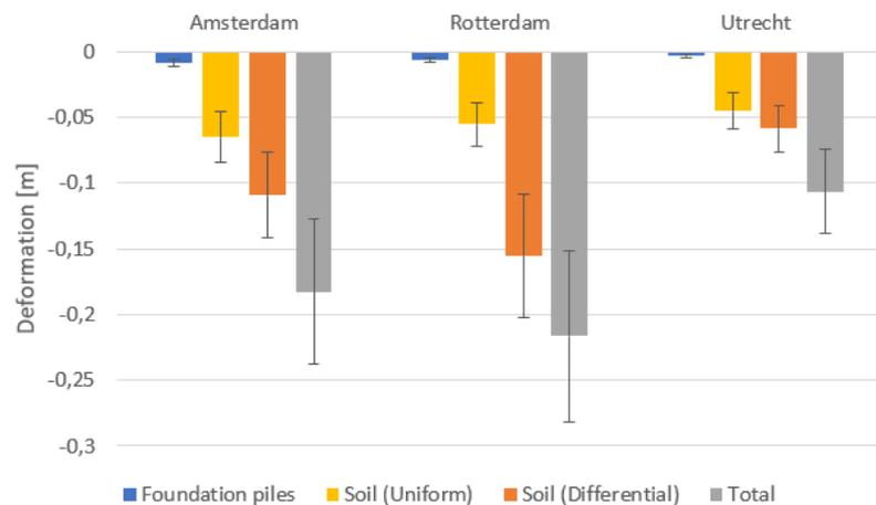
Figure 7.1: Components of the deformation for the concrete alternative
