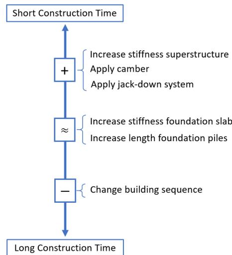
Figure 6.6: Ranking of the construction time of the mitigating measures
