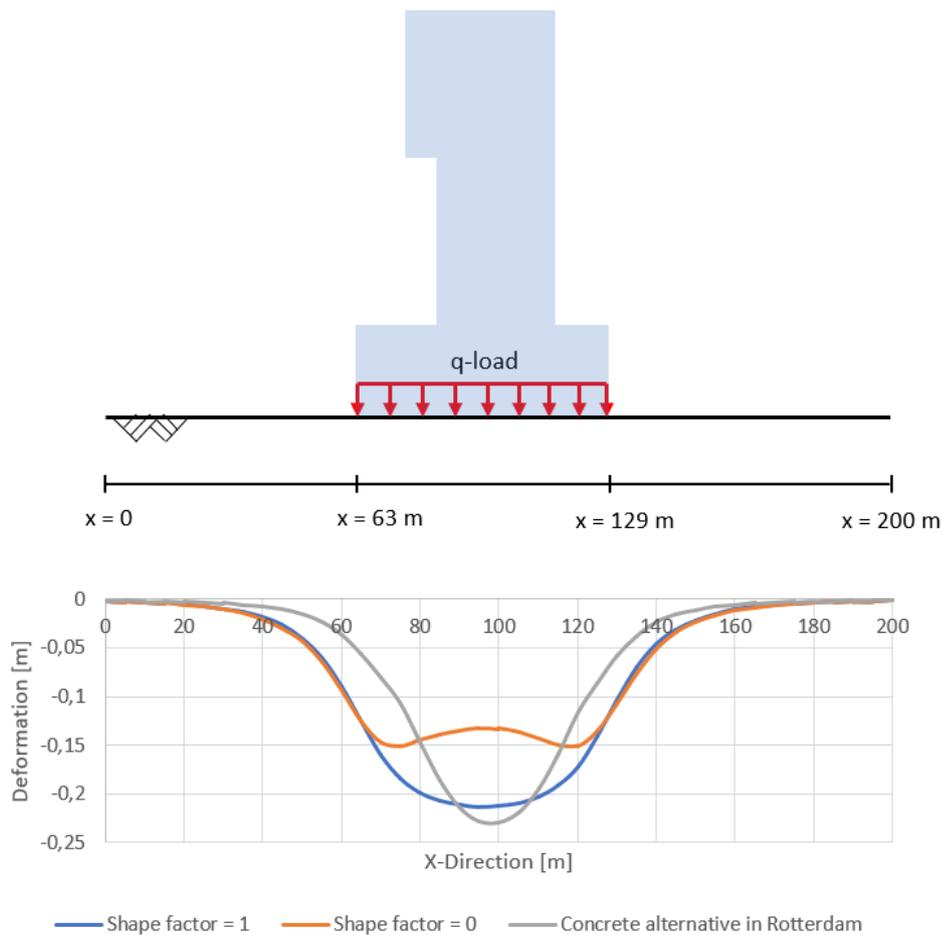
Figure 6.5: Results of the deformation of the soil for different load distribution to demonstrate the settlements of the building to the surroundings
