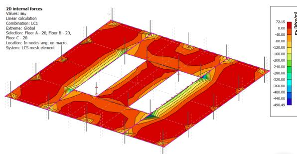
Figure A.11: Moment in x-direction in the concrete floor loaded in ULS
