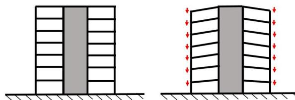
Figure 2.3: Schematic drawing of column shortening
