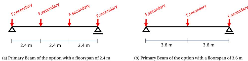
Figure A.15: Schematic drawing of the two options of the primary beam
