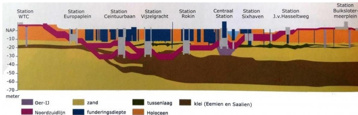
Figure 4.3: Cross section of the soil structure of Amsterdam [7]
