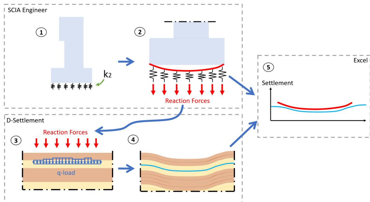
Figure 4.12: Overview of the method used to determine spring-stiffness  $k_2$
