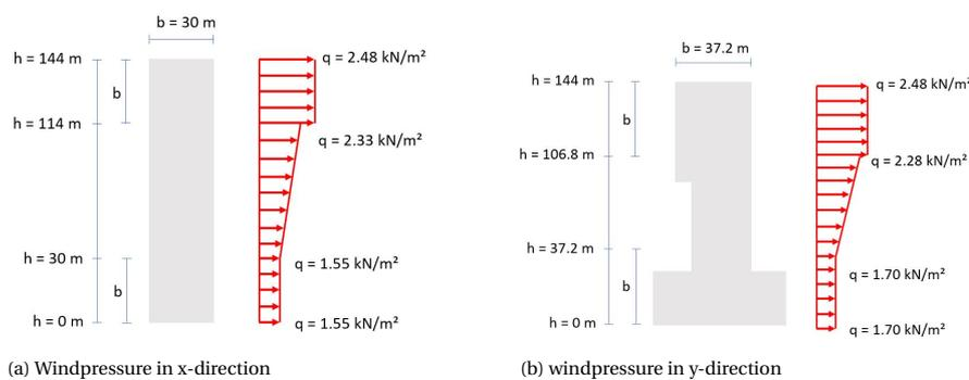
Figure 3.5: Windpressure on the building over the height
