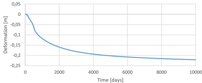
Figure 4.21: Deformation of the soil over time for the maximal deformation of the concrete alternative in Rotterdam
