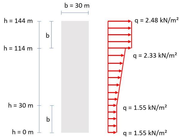
Figure A.6: Simplification of the wind pressure distribution over the height in x-direction
