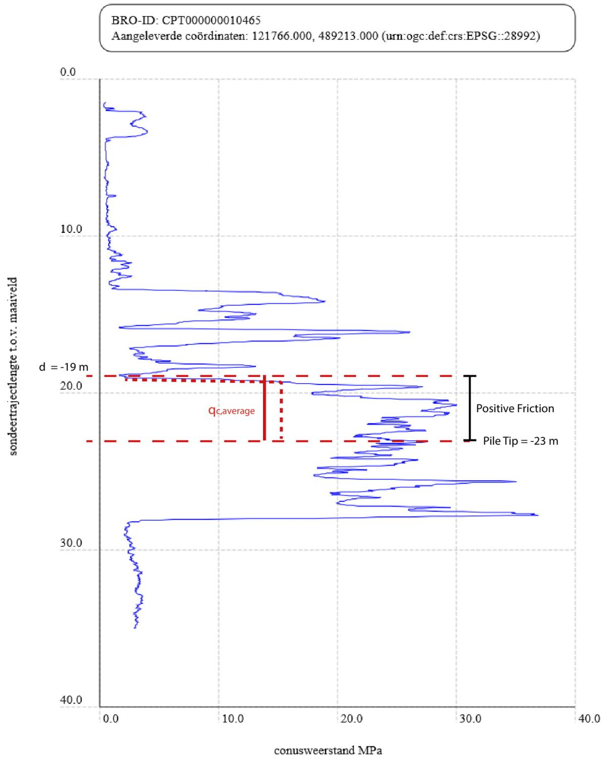
Figure B.2: Amsterdam - shaft friction resistance
