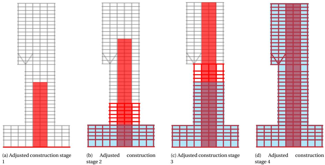
Figure 5.10: Adjusted construction sequence where the stability core is constructed in advance
