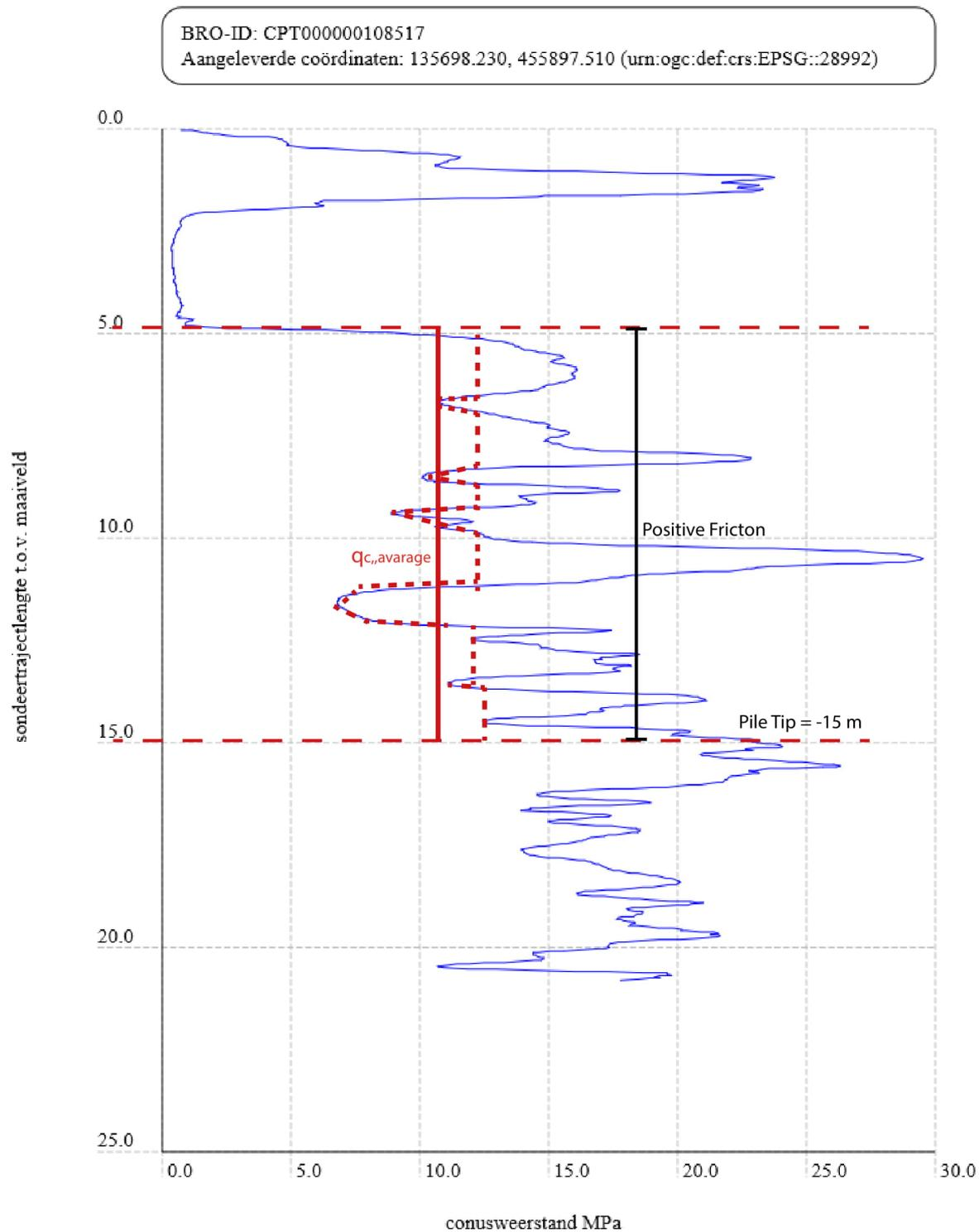
Figure B.6: Utrecht - shaft friction resistance
