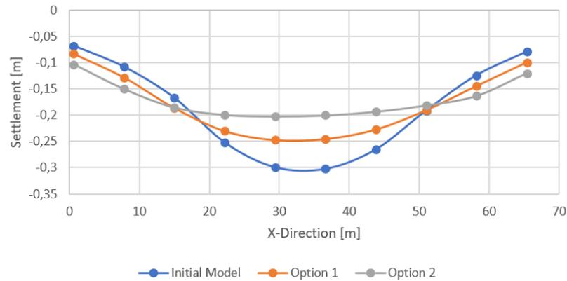
Figure 5.19: Graph of the deformation of the foundation slab for the different options of adding the diagonals
