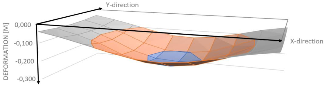
Figure 4.13: 3D view of the calculated deformation of the soil over the plot of the building for the concrete alternative in Rotterdam
