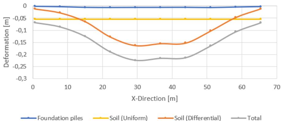
Figure 4.20: Components of the deformation in cross-section 1-1 for the concrete building at Rotterdam
