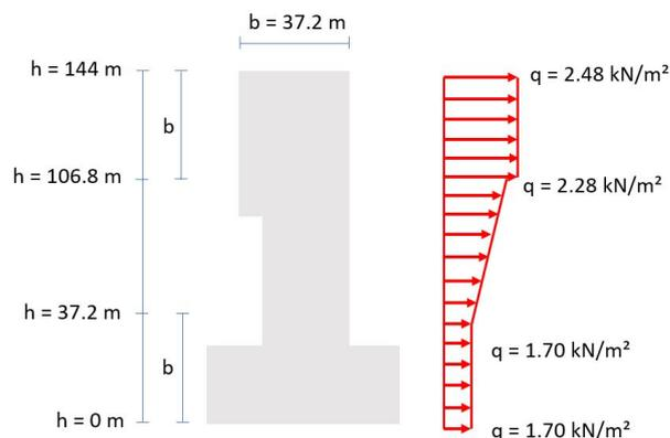
Figure A.7: Simplification of the wind pressure distribution over the height in y-direction
