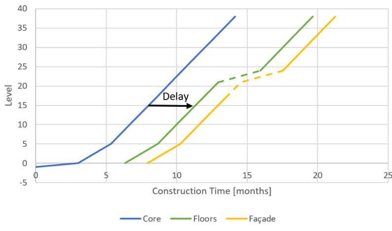
Figure 5.11: Height of the structure over time when the stability core is constructed in advance
