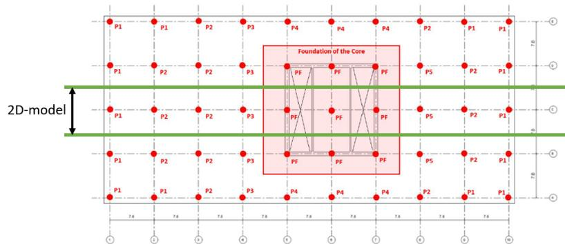
Figure D.1: Floorplan of the foundation floor with indicated which part of the structure is modelled in the 2D model.
