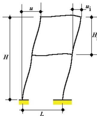
Figure 2.5: Definition of lateral deformation [6]
