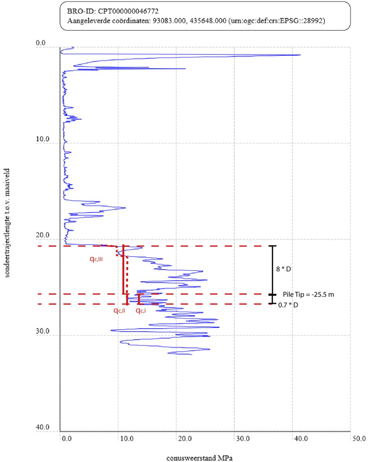
Figure B.3: Rotterdam - pile tip resistance
