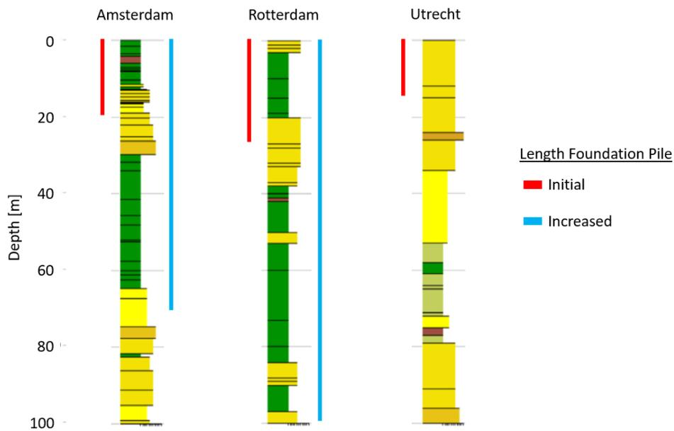
Figure 5.13: Schematic drawing to show the additional length of the foundation piles
