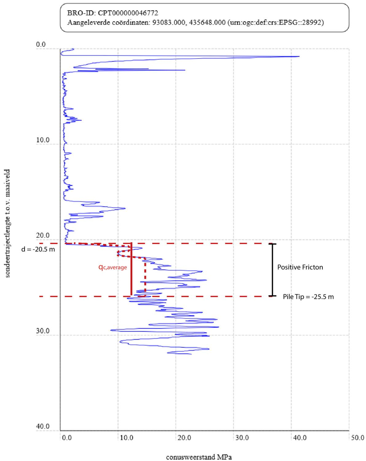
Figure B.4: Rotterdam - shaft friction resistance
