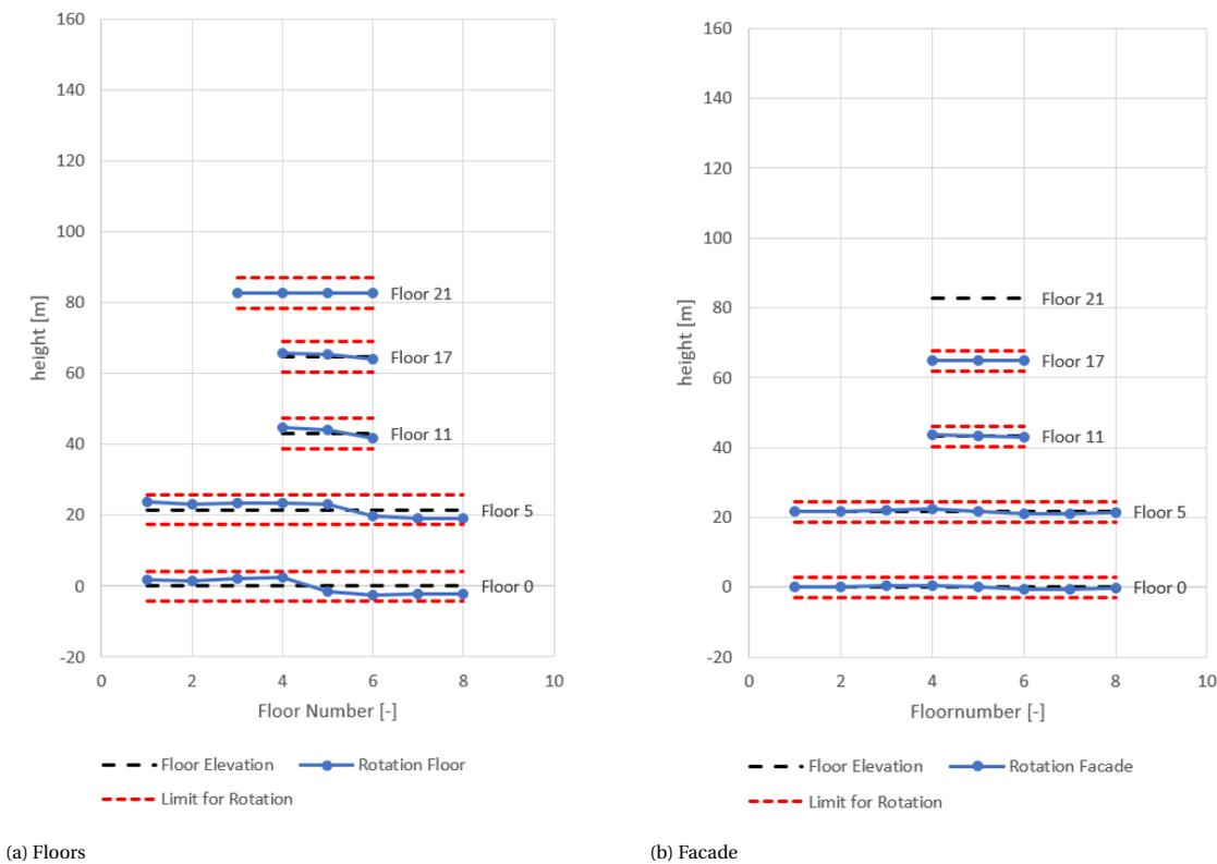
Figure 5.7: Deformation in construction stage 5 in cross-section 2-2 of the concrete alternative in Rotterdam
