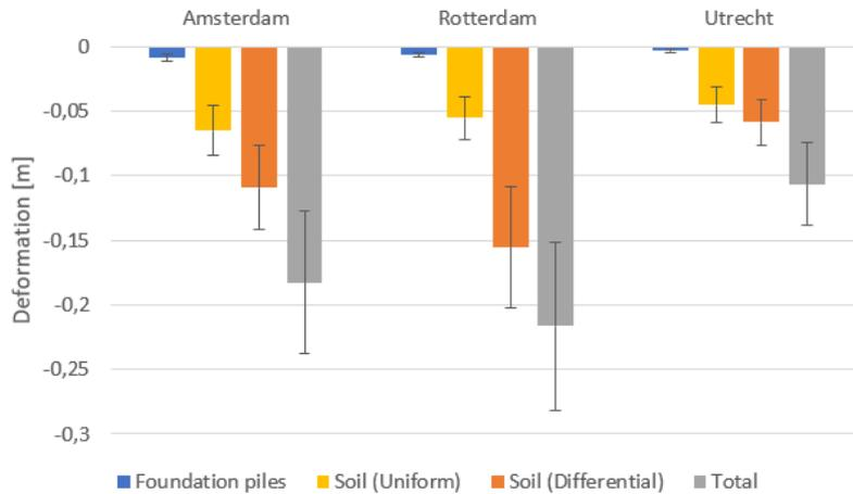
Figure 4.19: Components of the maximal deformation for the concrete alternative in Rotterdam
