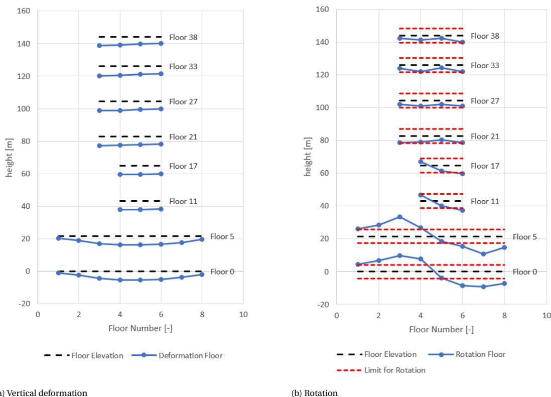
Figure 5.5: Final floor deformation in cross-section 1-1 of the concrete alternative in Rotterdam
