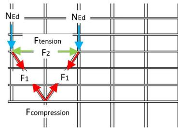
Figure A.16: Diagonals and tension beam
