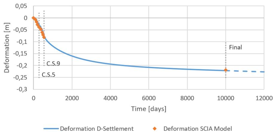
Figure 5.3: Time-dependent deformation of the soil compared to the deformation results in the SCIA model
