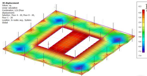
Figure A.12: Deformation of the concrete floor in SLS
