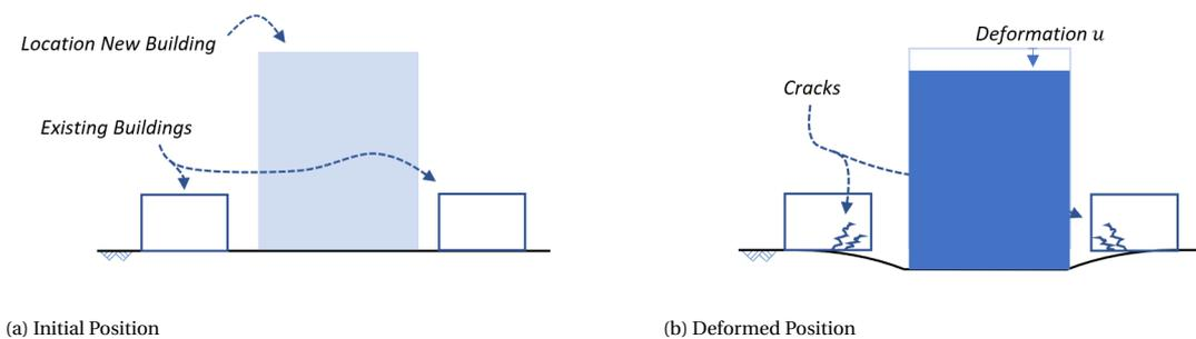
Figure 2.11: Schematic drawing to explain the problem for the adjacent buildings
