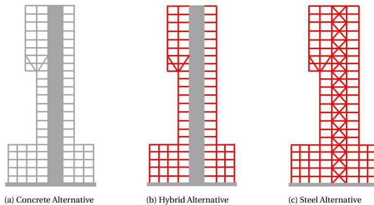
Figure 3.1: Schematic drawing of the three structural design for the building
