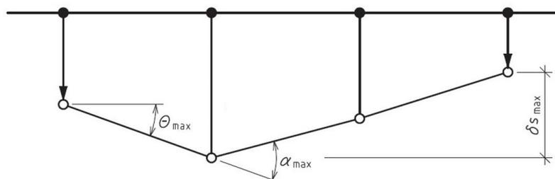
Figure 2.10: Definition of the relative rotation of the foundation [20]
