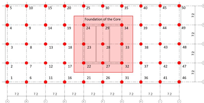
Figure C.2: The location of the foundation piles
