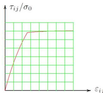
Figure 4.6: Loading of a over-consolidated soil [24]
