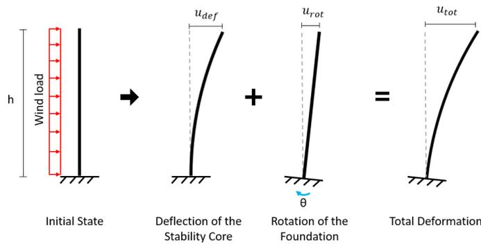
Figure 3.7: Deformation of the stability core under wind load
