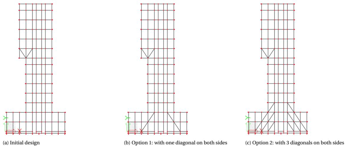
Figure 5.18: Schematic drawing of adding the diagonals to the structural design
