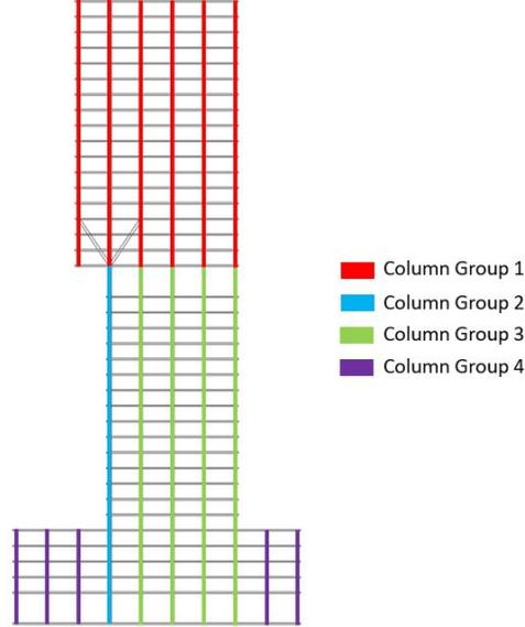
Figure 3.11: The column groups used to calculate the dimensions of the columns
