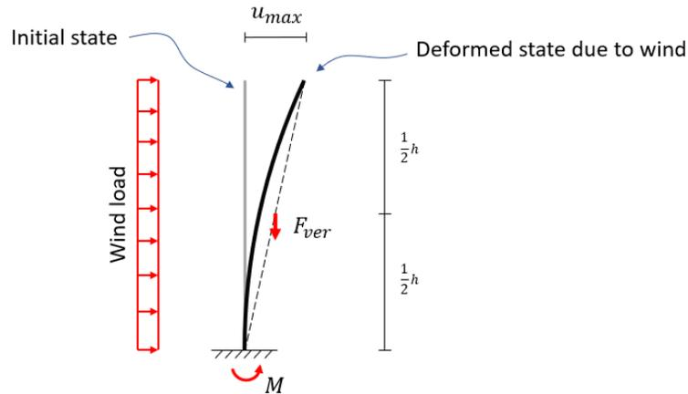
Figure 3.9: Deflection of the stability core
