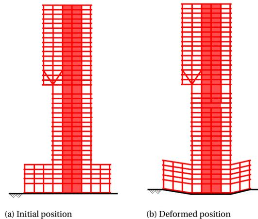
Figure 5.14: The deformation of the structure when the building is constructed without camber
