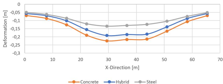
Figure 4.18: Results of the total deformation of the foundation slab in cross-section 1-1 of the three alternatives in Rotterdam without the error bars
