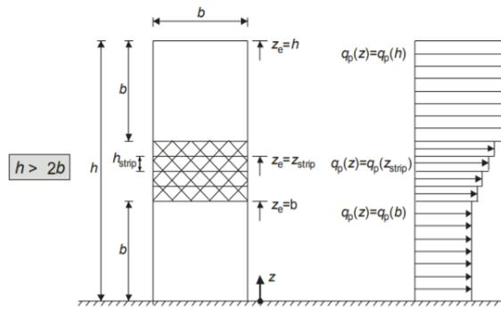
Figure A.5: Reference wind pressure over the height (Figure 7.4 in NEN1991-4) [19]
