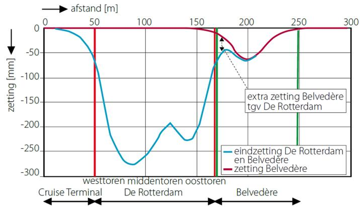
Figure 2.13: Calculated deformation of the soil for the building De Rotterdam [11]
