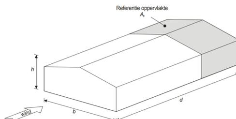
Figure A.8: Friction area of the wind on the building (Figure 7.22 in NEN1991-4) [19]
