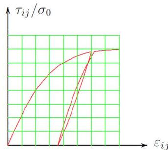
Figure 4.4: Loading and unloading of soil [24]
