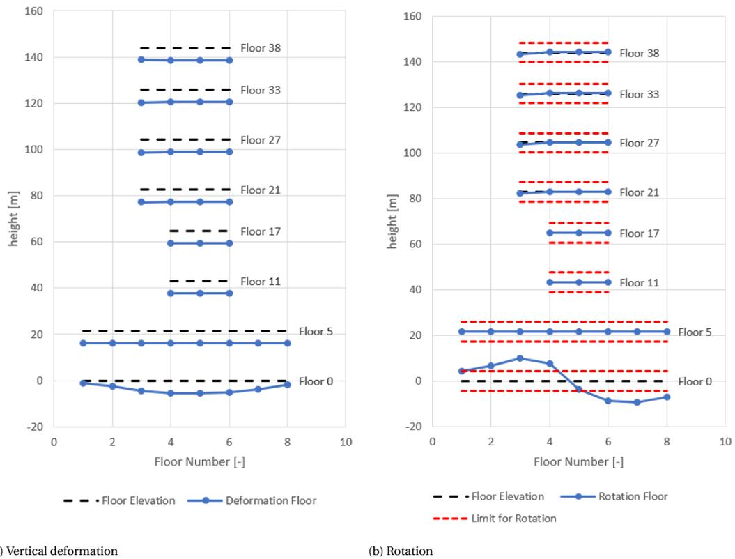
Figure 5.22: Final floor deformation for the structural system with jack-down system in cross-section 1-1 of the concrete alternative in Rotterdam
