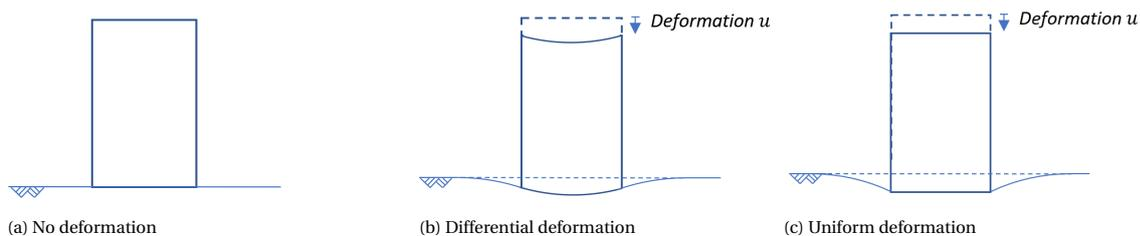
Figure 6.4: Schematic drawing to explain the options of deformation of the soil
