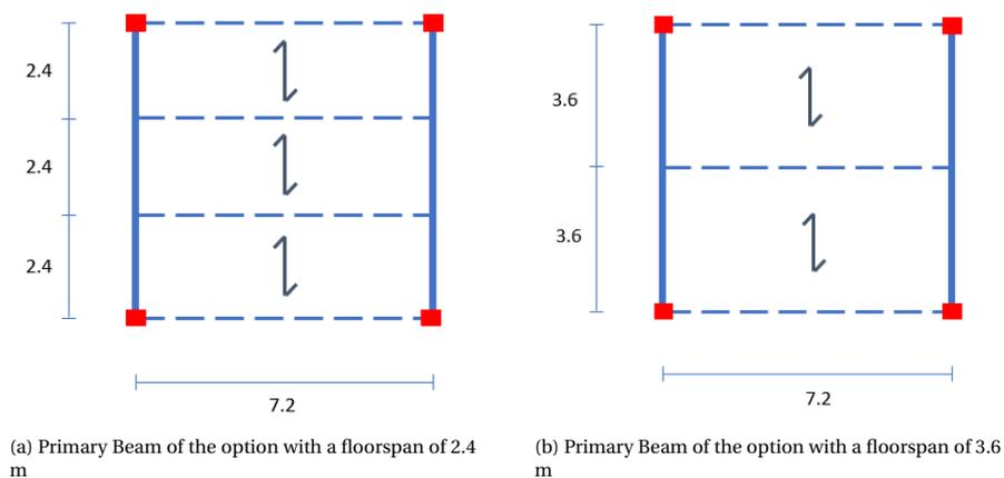
Figure A.14: Topview of the two options considered for the lightweight floor for the steel alternative
