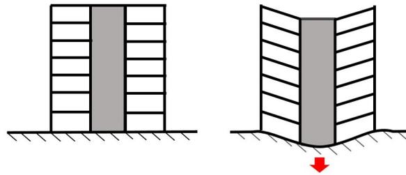
Figure 2.2: Schematic drawing of deformation of the foundation
