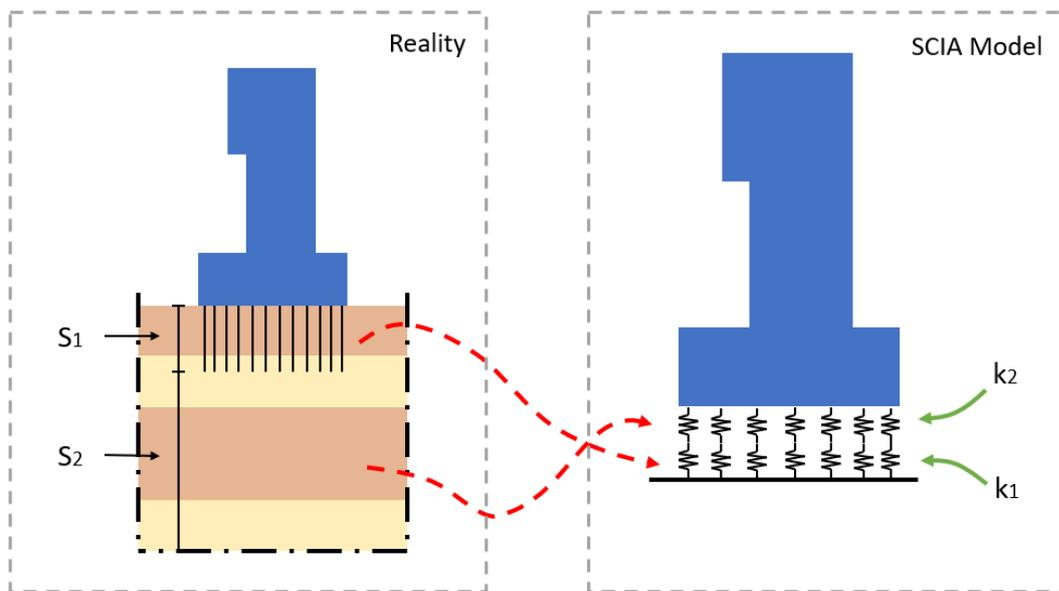
Figure 4.9: Schematic drawing of how the reality is modeled with the consecutive springs in the SCIA model (the springs are swapped compared to the reality in order to simplify the model)
