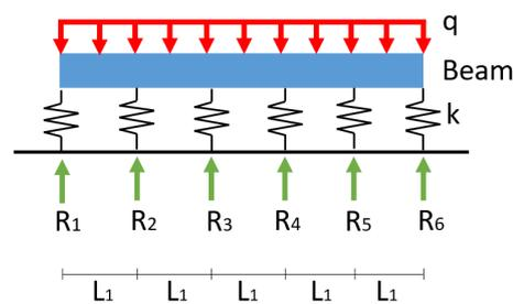
Figure 4.7: Example structure to explain the change in reaction force
