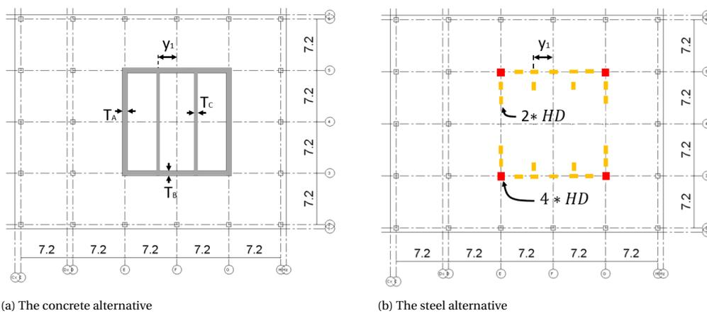
Figure 3.8: Horizontal cross-section of the stability cores
