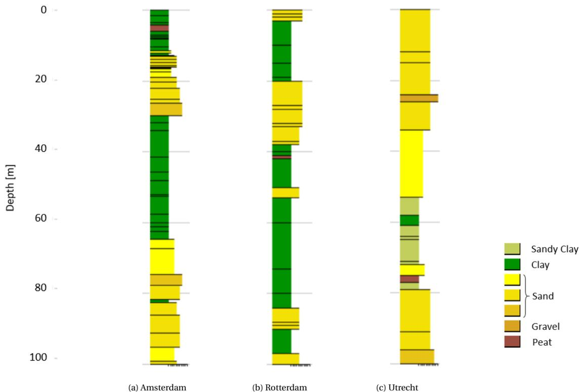
Figure 4.2: Soil structure per location
