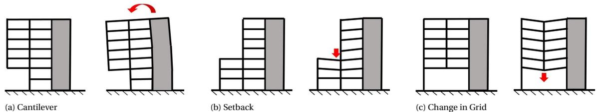
Figure 2.4: Schematic drawing of discontinuities in the geometry
