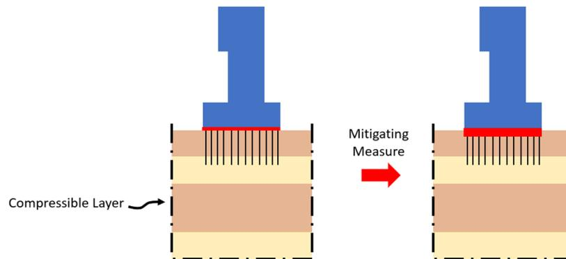
Figure 5.16: Schematic drawing of increasing the thickness of the foundation slab
