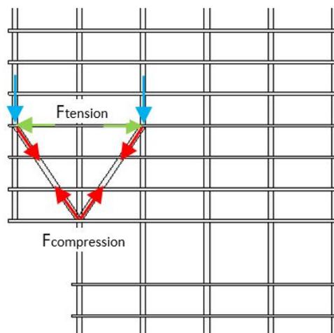
Figure 3.12: Diagonals and tension beam which support the cantilevering part of the building
