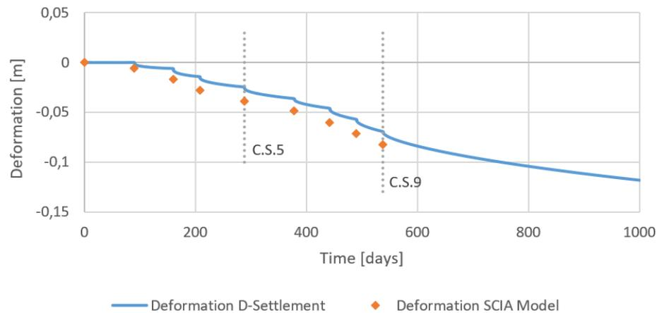
Figure 5.4: Detail of the time-dependent deformation of the soil compared to the deformation results in the SCIA model
