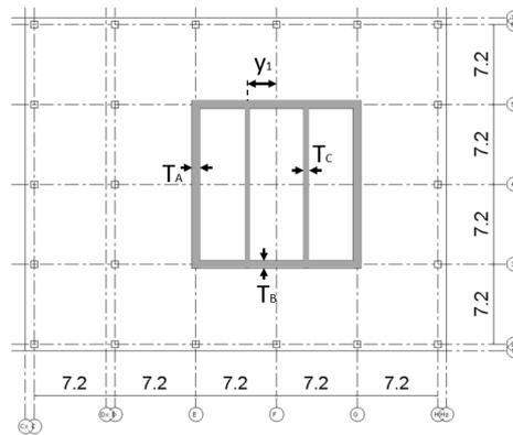
Figure A.9: Horizontal cross-section to show the concrete core
