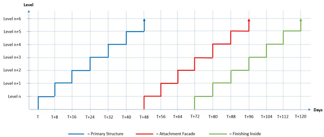
Figure 3.15: Construction sequence for a typical floor in the high-rise part of the building
