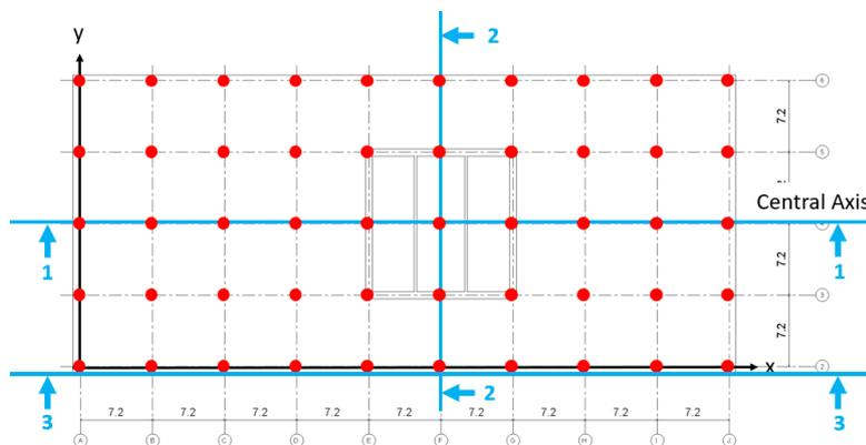
Figure 4.10: Top-view of the foundation floor with the locations of the supports and the considered cross-sections
