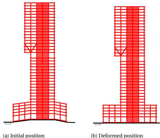
Figure 5.15: The deformation of the structure when the building is constructed with camber
