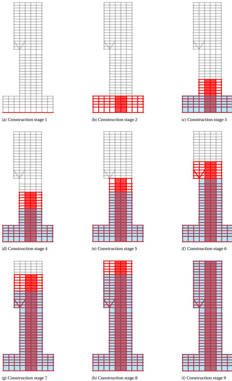
Figure 5.2: Assumed construction sequence used for the structural analysis
