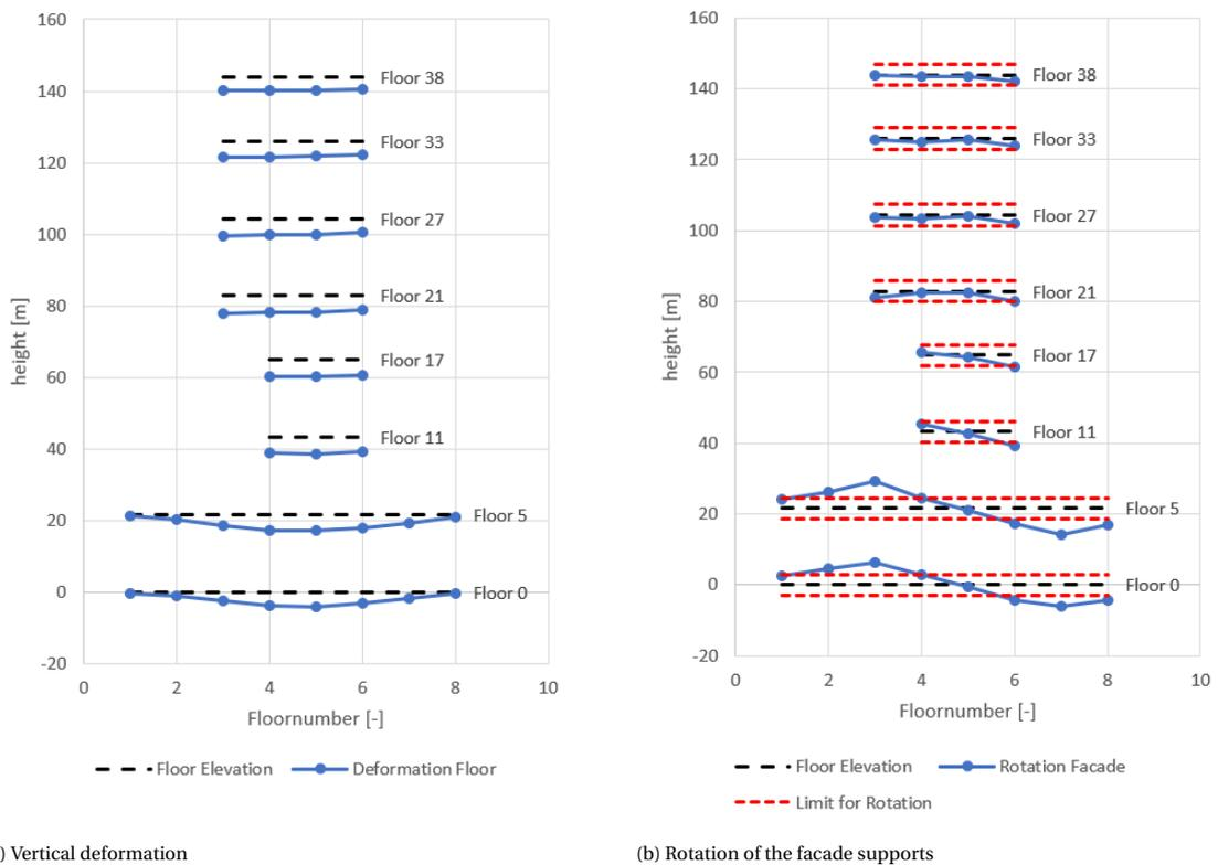
Figure 5.6: Final facade deformation in cross-section 2-2 of the concrete alternative in Rotterdam
