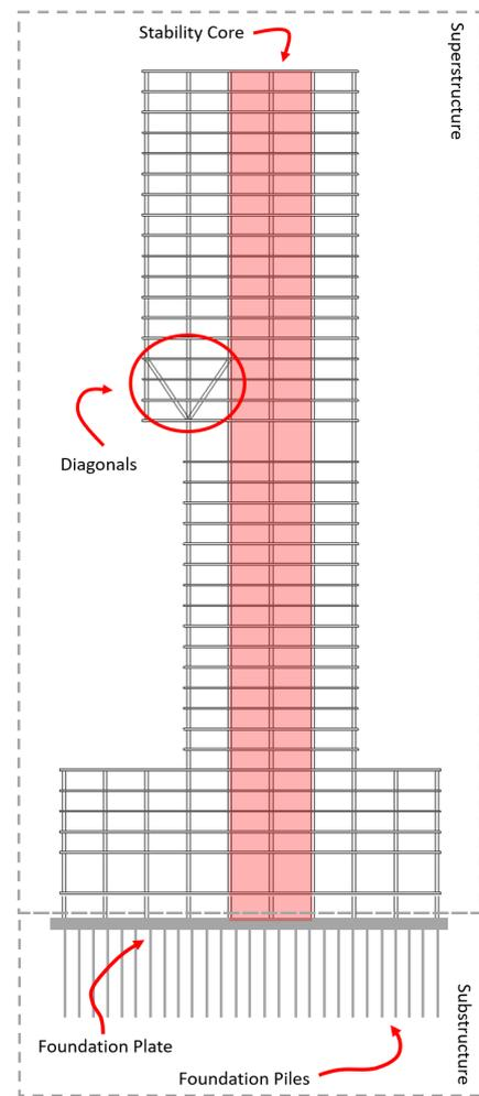
Figure 3.6: Schematic drawing of the structural system
