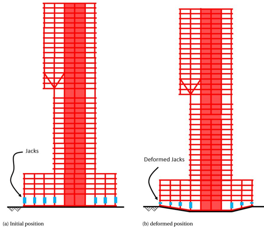
Figure 5.21: Schematic drawing of the jack-down system in the structure
