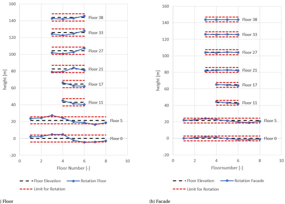
Figure 5.8: Deformation in construction stage 9 in cross-section 2-2 of the concrete alternative in Rotterdam
