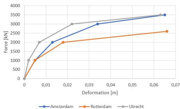
Figure 4.11: Load-settlement curve of the foundation pile per location
