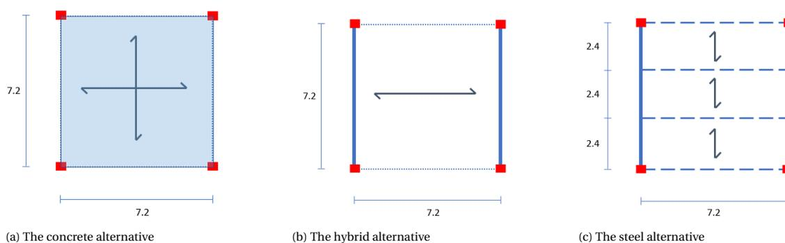
Figure 3.10: Floor systems for the different alternatives
