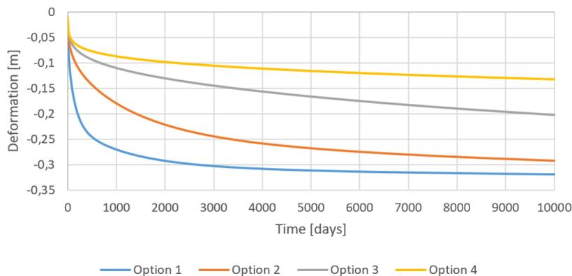
Figure 5.9: Deformation of the soil over time for the 4 options in Rotterdam
