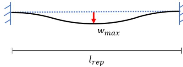
Figure 2.8: Schematic drawing of the deformation of the floor system
