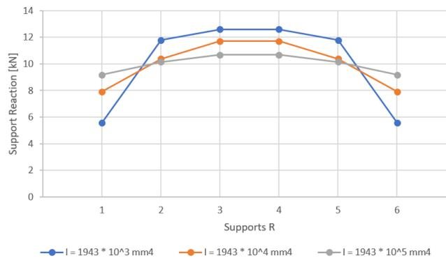
(b) Stiffness of the structure (stiffness soil is 1 MN/m)
