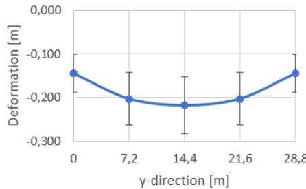
(b) Deformation of the soil in cross-section 2-2
