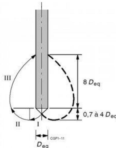
Figure 3.14: Trajectories of the method of Koppejan [1]
