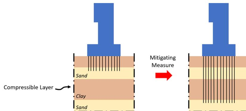
Figure 5.12: Schematic drawing of increasing the length of the foundation piles to the second sand-layer
