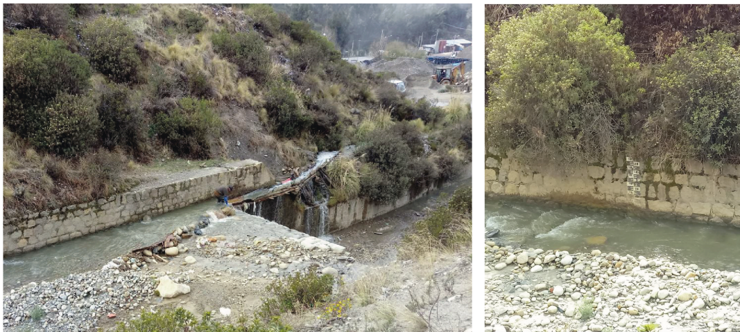
Figure 2.1: Two problems related to discharge and its data. The photo on the left shows an illegal intake, located before the measurement location. The photo on the right shows the stage scale, on which the scale has faded. Both images are made- and provided by Harm G. Nomden, photos are taken in 2017.
