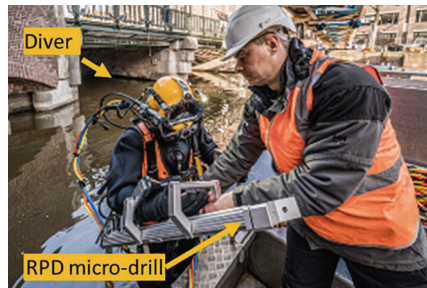
Fig. 10. RPD deployment underwater by a diver.
