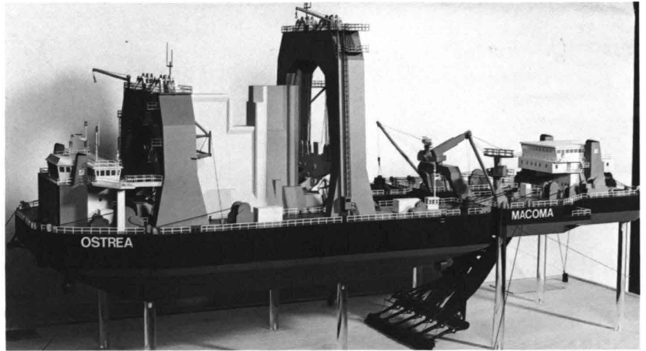
11 Ostrea/Macoma combination for installing the piers and dredging sand deposits
