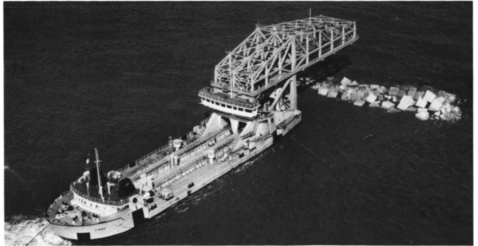
5 Stone dumping barge at Rotterdam harbour entrance
