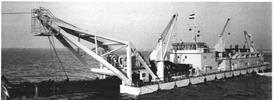
3 Cutter suction dredger
