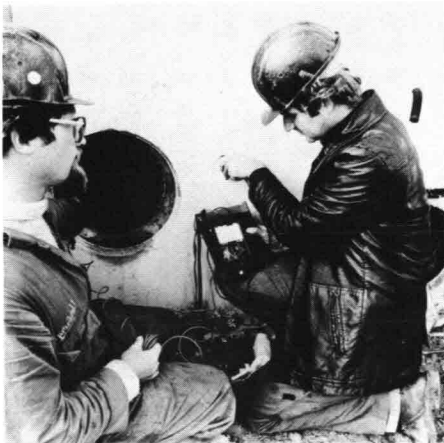
15 Control measurement electrical resistance anchor bolt
