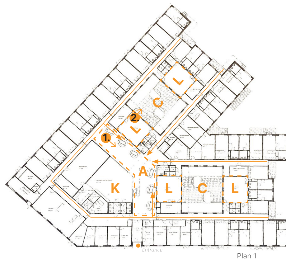
Figure 36. Ground floor plan, Yulius, showing the functions and organization
