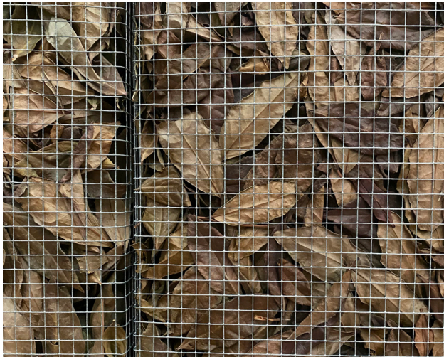
Figure 41. Closeup look at the gabions filled with tea leaves
