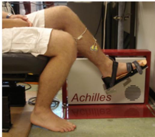
**Figure 2-1: Measurement Set Up.** The foot of the subject was fixated to the Achilles foot plate such that the rotation axis of the ankle was aligned with the axis of the manipulator. Joint angle, velocity, torque and EMG of plantar flexor and dorsiflexor muscle were measured.
