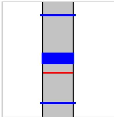
**Figure 2-5: Active RoM screen.** Feedback screen during Active RoM. The blue square in the centre represents the ankle position where the foot is perpendicular to the lower leg ( $0^\circ$ ). The thin blue lines are the maxima of dorsi- and plantarflexion achieved during that trial, these lines move when a larger angle is achieved. The red line shows the current position.
