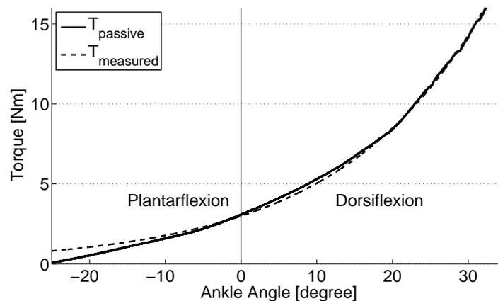
**Figure 2-3: Identification.** Example of measured ( $T_{measured}$ ) (dotted) and modeled ( $T_{passive}$ ) (solid) passive relation between ankle angle and torque. The modeled torque was obtained by minimization of least square error between the measured and the modeled torque. All relations are modeled from zero torque to full dorsiflexion.
