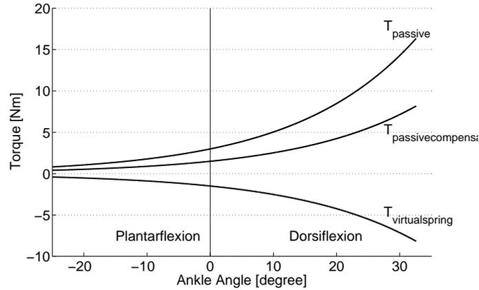
**Figure 2-2: Stiffness compensation.** Simulated passive stiffness compensation for  $\alpha=-0.5$ . In the case of negative stiffness compensation the angle-torque relation,  $T_{passive}$ , is lowered by the torques created by the virtual spring,  $T_{virtualspring}$  resulting in an altered angle-torque relation  $T_{passivecompensated}$ .
