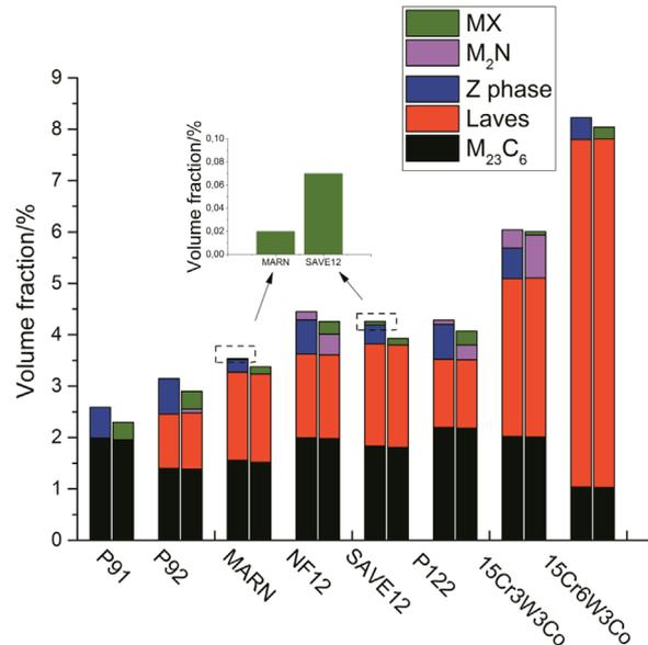
**Figure 4.** The calculated equilibrium precipitate populations (columns on left) and the precipitate populations with Z-phase being computationally suppressed (columns on right) for heat resistant steels.
