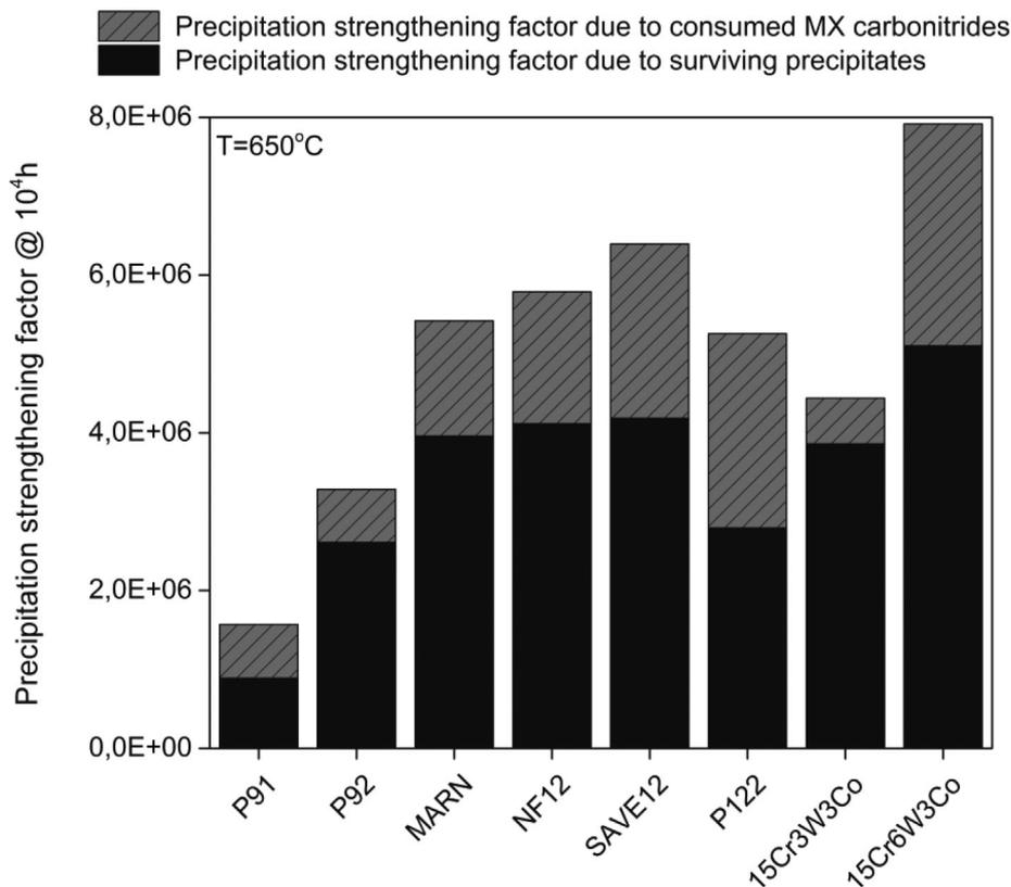
**Figure 5.** The calculated precipitation factor after 10<sup>4</sup> h due to the surviving precipitates (M<sub>23</sub>C<sub>6</sub> + Laves phase) and the MX carbonitrides to be consumed in the Z-phase formation.
