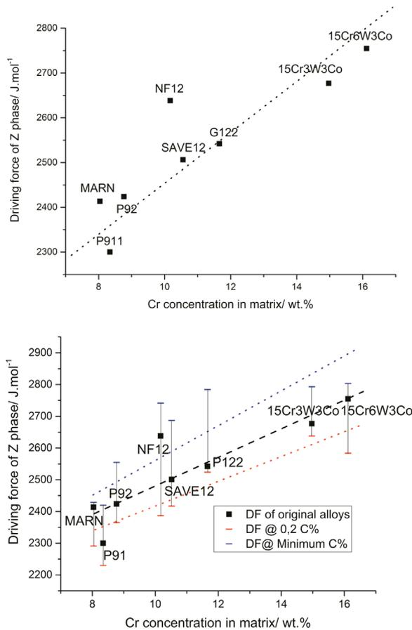
**Figure 6.** The calculated driving force for Z-phase formation in exiting heat resistant steels (in black dash line), as well as the calculated upper and lower limit of Z-phase driving force with specification permitted C concentration differences (in blue and red dot lines), as a function of Cr concentration in matrix as at 650 °C.
