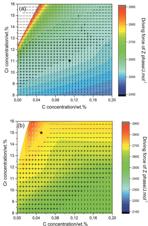
**Figure 7.** The binary isopleths of C–Cr for the calculated driving force of Z-phase in commercial grades a) P122 and b) 15Cr6W3Co steels. The black star symbols show the nominal concentration values for the P122 and 15Cr6W3Co alloys, respectively.
