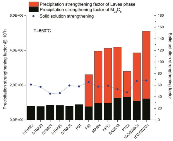
**Figure 2.** The calculated precipitation strengthening factor of  $M_{23}C_6$  and Laves phase in existing Cr containing steels, at the temperature of  $650^\circ\text{C}$  and service time of  $10^4\text{h}$ ; and the calculated solid solution strengthening factor of existing Cr containing steels.
