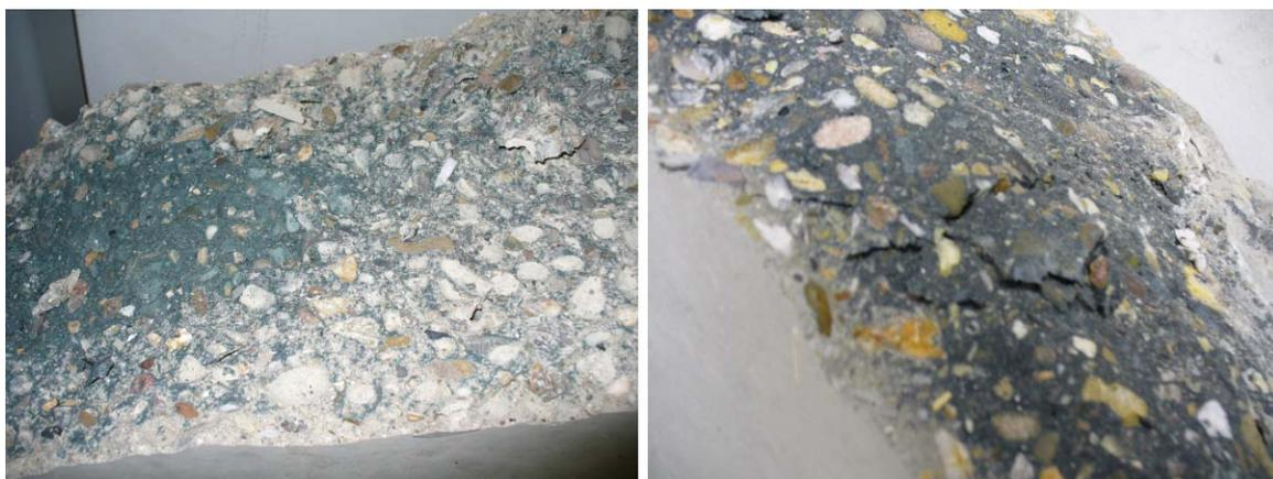
**Fig. 23: Surface of crack in NSC (Left) and HSC beam (Right)**
