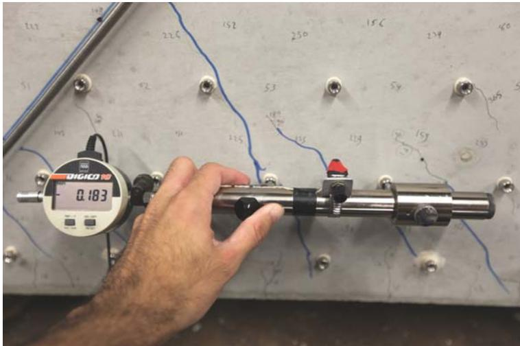
**Fig. 13:** Measuring of the distance between the points by means of a hand-operated LVDT
