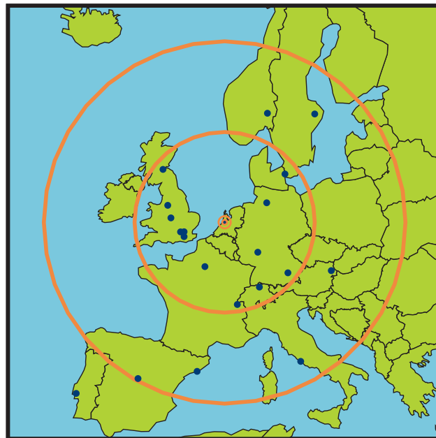
Figure 1.2: Proximity of origin airports in Europe: The map shows the 20 busiest connections into Amsterdam Airport Schiphol in 2013 according to [21]. The range rings indicate 400 and 800 nautical miles or one and two hours flight time, respectively.
