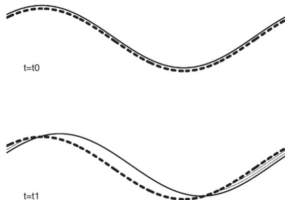
**Figure 3.4:** Illustration of Pipe Exposure due to Sand Waves Migration: Dotted line represents sand wave profile and solid line represents pipe alignment [28]
