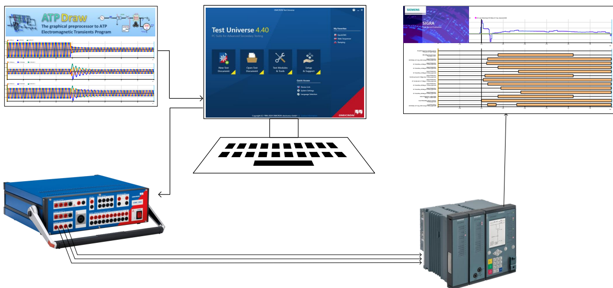
Figure 6.1: Hardware testing setup
