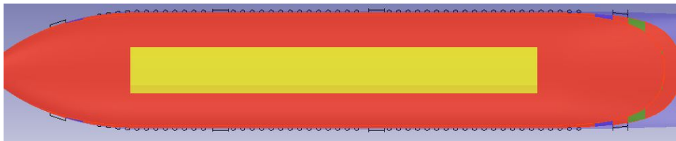
Figure 2.19: Bottom view of a Prandtl Plane with 248 passengers and a continuous cargo hold
