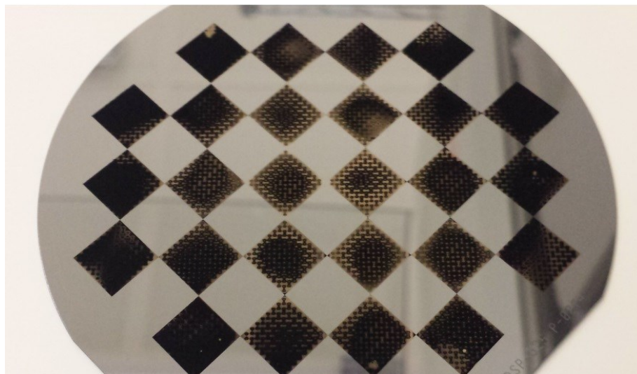
Figure 7.8: Image of the bottom wafer showing a reverse loading effect. The growth has been more towards the periphery compared to the center.
