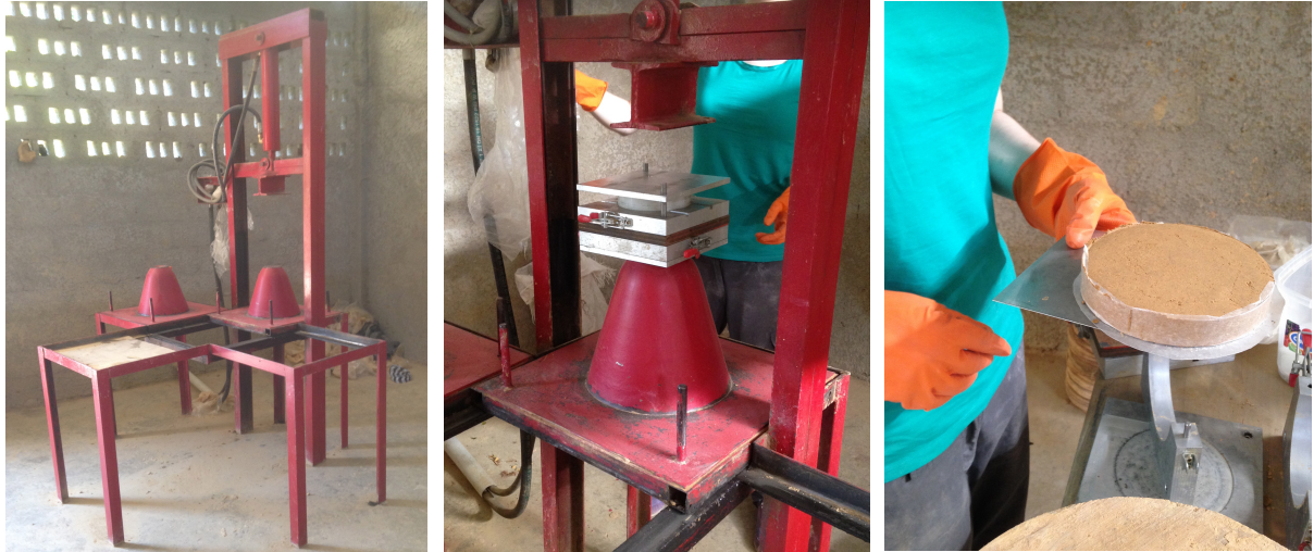
Figure I-2 | Pictures of the manufacturing proces of the CDFs. From left to right: the press to press the CDFs, the press together with the mold and a pressed CDF.
