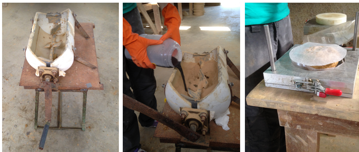
Figure I-1 | Pictures of the manufacturing proces of the CDFs. From left to right: the mixer with which the clay mixture was mixed, the addition of a metal solution to a dry clay mixture and a clay ball inside the mold.
