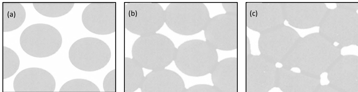
Figure 2-7 | The development of the ceramic structure during vitrification: (a) loose clay particles, (b) initial stage of vitrification and (c) intermediate stage of vitrification.
