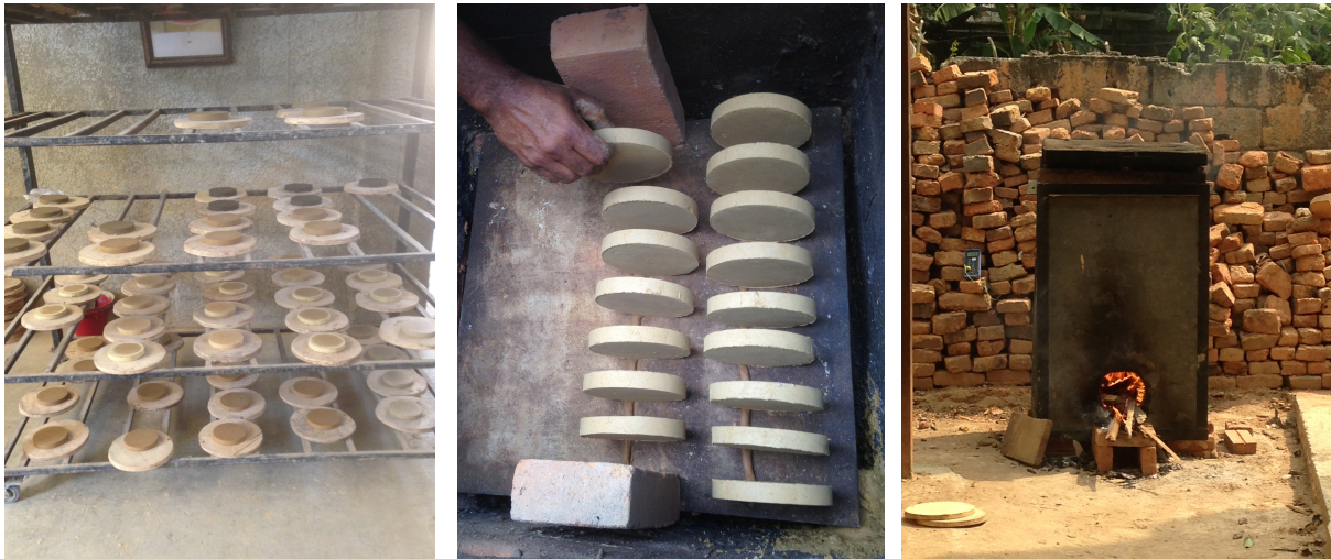
Figure I-3 | Pictures of the manufacturing proces of the CDFs. From left to right: CDFs that are drying, CDFs inside the kiln and the kiln with which the CDFs were fired.
