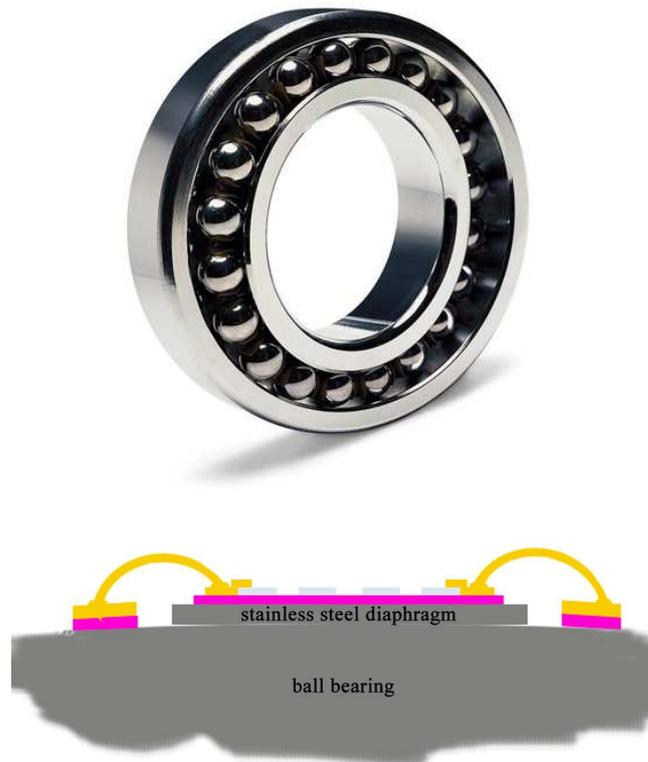
Figure 1.1: Ball bearing and expected bearing-scale fabrication cross section
