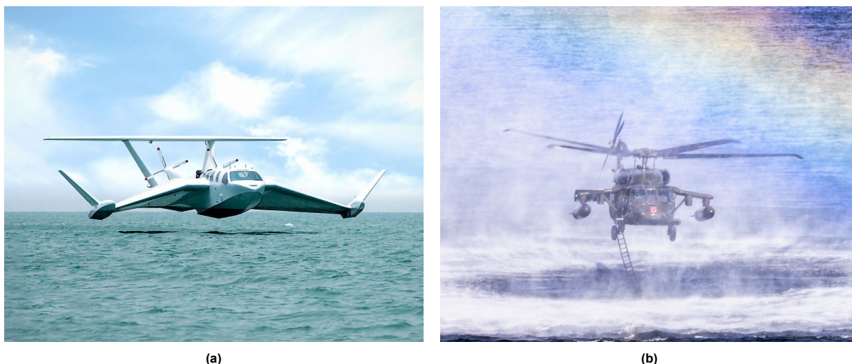
Figure 1.2: Examples of vehicles operating in ground effect: (a) a modern ekranoplan exploiting lift augmentation [4]; (b) a helicopter experiencing modified induced flow during hover [5].
