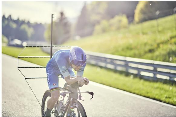
Figure 2.7: Patrick Lange track test with the *SwissSide* pressure rake at the Salzburgring race track (Dirksen, 2019).
