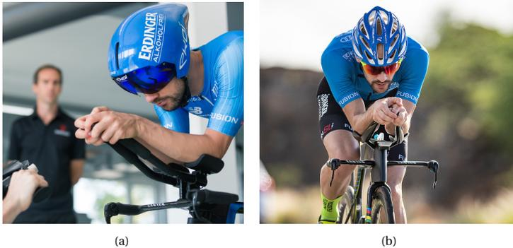
Figure 1.3: (a) Baseline extension bar setup, with existing gap (Hilger, 2018). (b) Innovative 3D printed aerobars, individually shaped to fit the cyclist's arm (Rauschendorfer, 2018).
