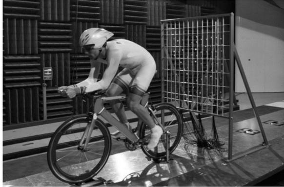
Figure 2.5: Single rider setup with a pressure wake rake 600mm downstream of athlete. (Barry, 2015)
