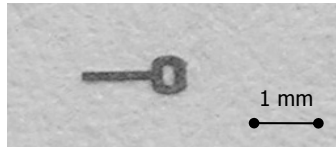
Figure 2-5 Drive pin for a micro-loud speaker, assembled semi-automatically
