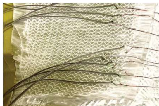
(b) Soldered wiring embedded in glass fiber laminate.
