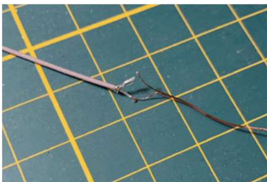
(a) Result of soldering copper to coax wire.
