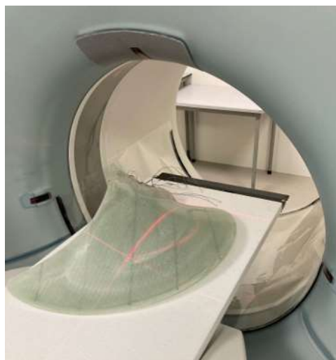
(a) Macro CT machine with FRC blade.
