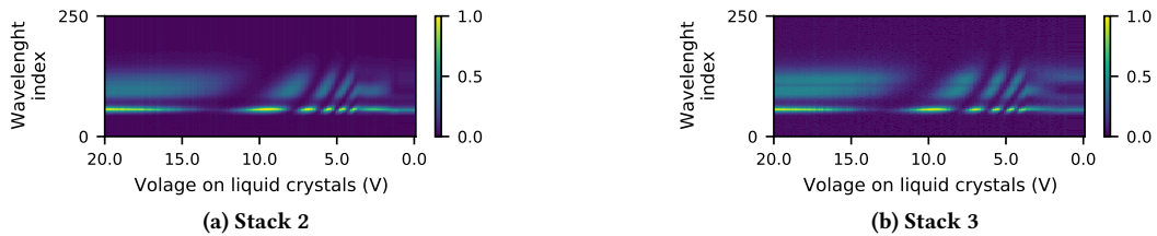
Figure 15: Characterization of different stacks of LCs. Apart from the unstable region in low voltages, the patterns are the same.
