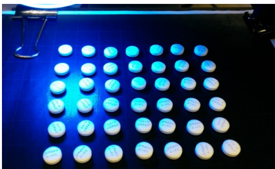
Fig. 7. Arrayed tablets. We can keep the ground truth of individual tablet IDs between the first (database) and the second (query) turns of image collection.
