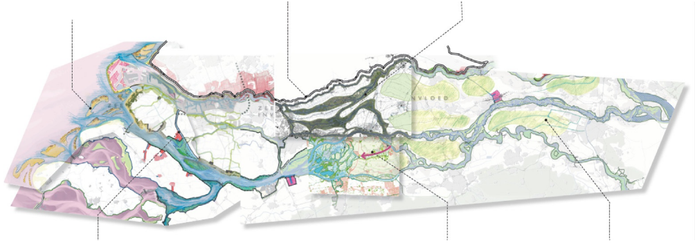
Fig. 4 Design study exploring the Haringvliet estuary as the new main discharge channel of Rhine and Meuse, reducing the role of the New Waterway in the discharge distribution. Design by H+N+S Landscape Architects, commissioned by the Dutch Delta program, 2012.
