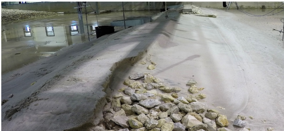
Fig. 2 Photo of 3D wave basin experiment on wave overtopping of sand-covered rubble-mounds at Texas A&M University's Haynes Laboratory.
