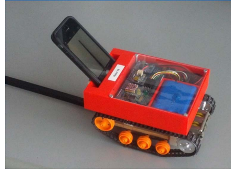
Fig. 4. Diagram of line-follower robot
