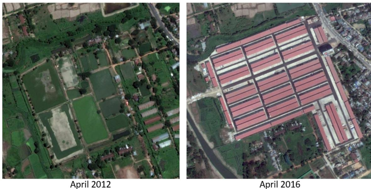
Fig. 6.8: Before and after images for the construction of a compound for which a surface deformation velocity of 4 cm/y downwards was measured. This structure is located at 16°55'27" N and 96°9'31" E.
