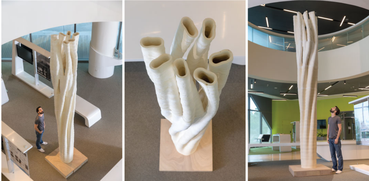
Figure 1. 3-d printed mould made with fungal-like adhesive materials (FLAM), credits: Fernandez (2019)
