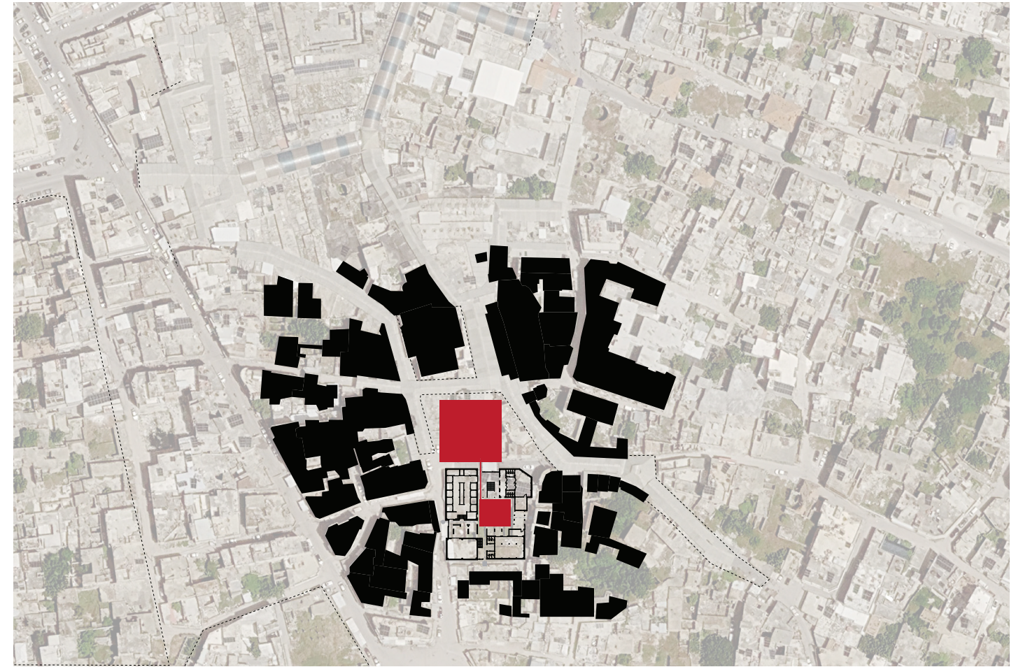
Figure 11 | Close-up interpretation of the selected building block within the zoomed-in urban plan. This drawing explains how the selected intervention area relates to the surrounding bazaar fabric, urban pockets, access routes, and nearby public spaces. At this scale, the masterplan strategy becomes more specific, showing how the building block can act as a public-economic node while connecting to the wider recovery plan of the Old Town.
