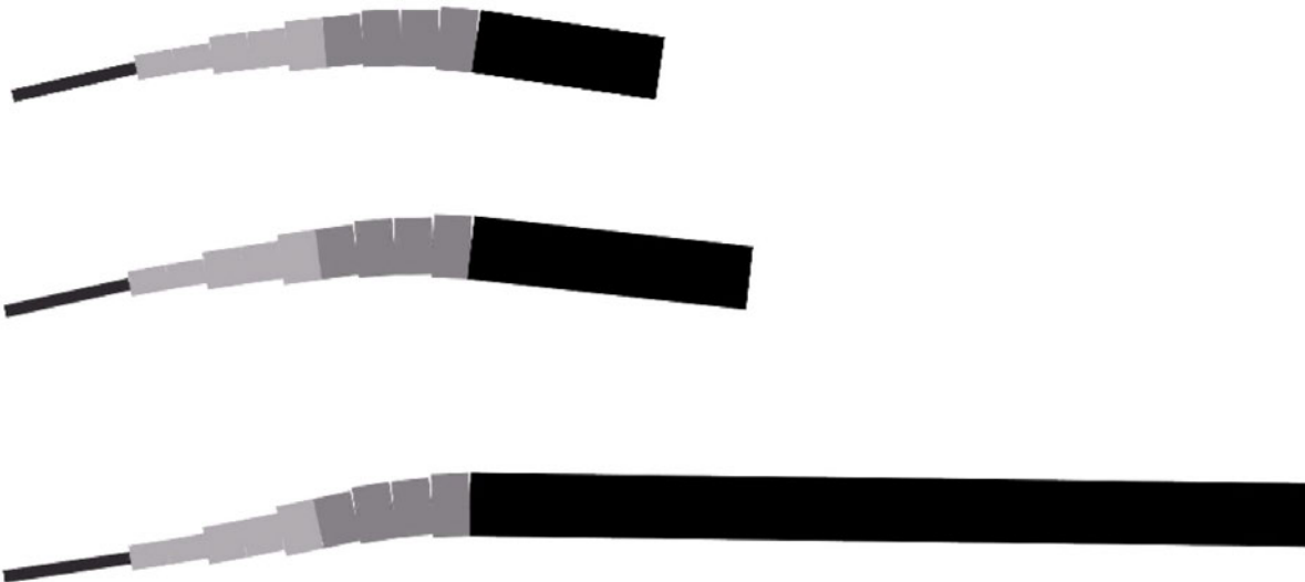
Figure 5.5: The center of rotation is placed at the center of mass of the complete body the rigid head is \frac{1}{3} , \frac{1}{2} and \frac{3}{4} of mass of the total body. Black on the right is the passive head, dark grey active tail, light grey passive tail, black on the left, the caudal fin. Screenshot is taken at the maximum tail amplitude. Video: https://youtu.be/oxUJU0yoq6w
