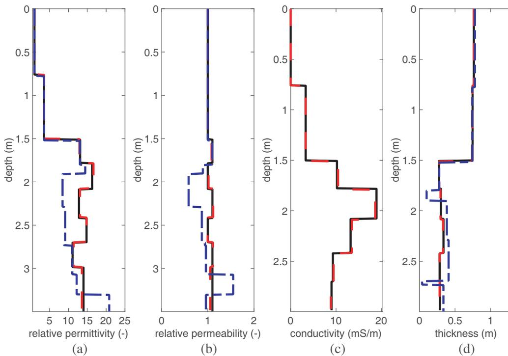
**Figure 4.** The comparison with the Marchenkon inversion values (red dashed-dotted lines), the direct inversion values (blue dashed-dotted lines) and the model values (solid black lines): (a) relative permittivity; (b) relative permeability; (c) conductivity; and (d) thickness.
