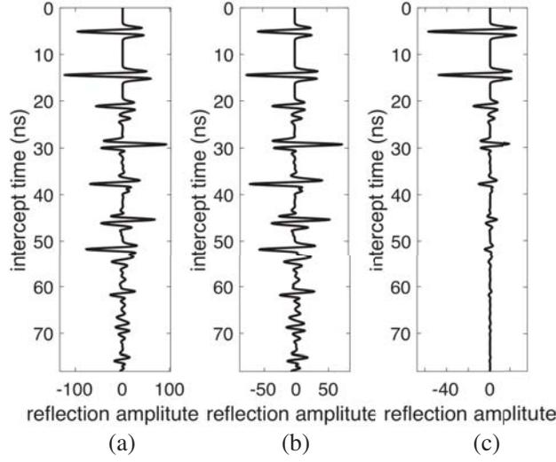
**Figure 2.** One trace ( $p = 0$ ) for the reflection response: (a) in the dissipative medium, (b) in the effectual medium, and (c) in the lossless medium. The black arrows indicate the primary reflections.
