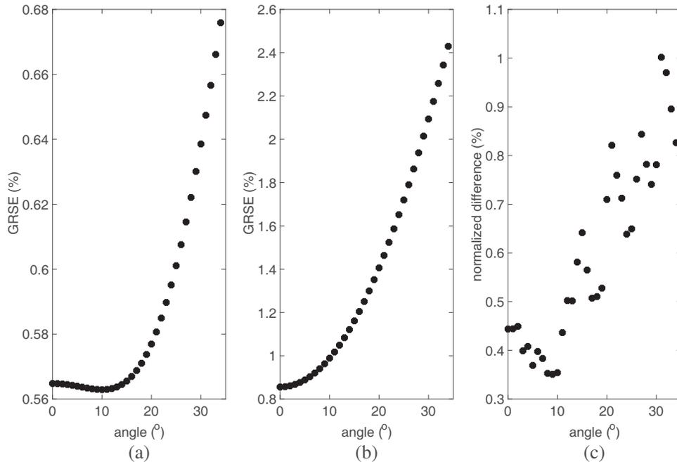
**Figure 5.** The GRSE of the retrieved dataset for different incidence angles: (a) the GRSE of up-going wave fields received on the surface, (b) the GRSE of transmission data received on the bottom, and (c) The relative errors of the reflection coefficients as a function of  $p$  for the 3th reflector in the lossless medium.
