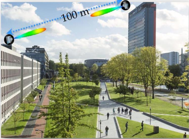
Figure 1.5: TU Delft envisioned 170 GHz point to point link based on the Fly’s Eye concept, providing the test case for the specifications of this project
