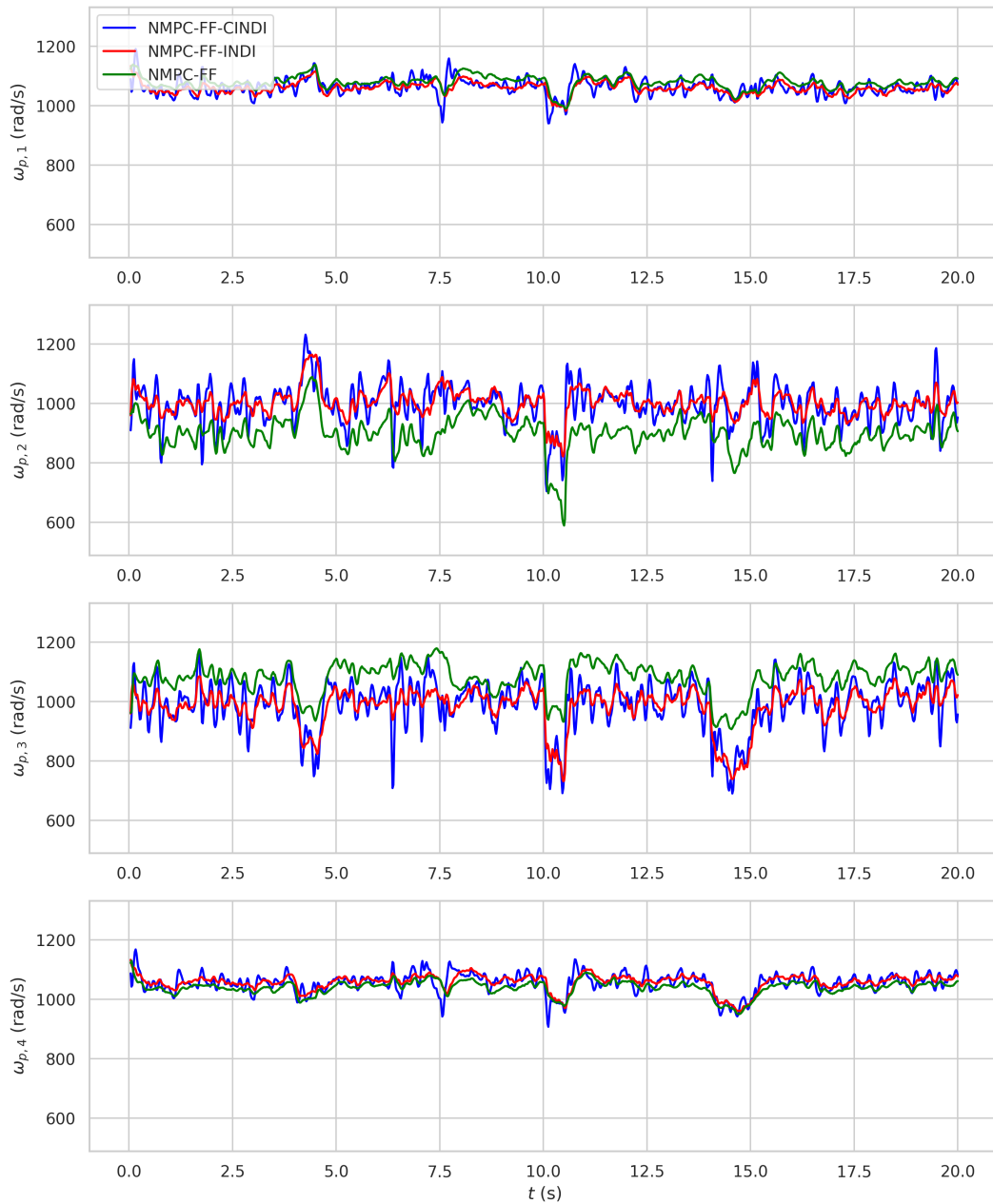
Figure 5-6: The commanded propeller speeds during the eight-like free flight experiment with disturbances.
