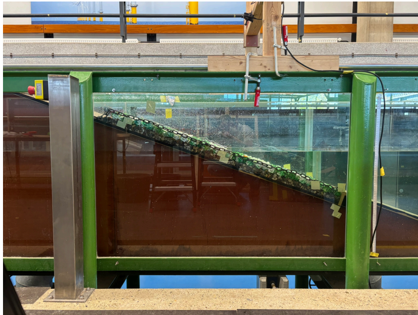
Figure 3.4: Side view of the as-built model with \cot \alpha = 3 slope and t_f = 1.0 D_n quarry-stone underlayer, photographed through the glass sidewall of the flume.
