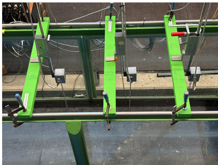
Figure 4.2: The three resistance-type wave gauges in the flume, mounted seaward of the structure.
