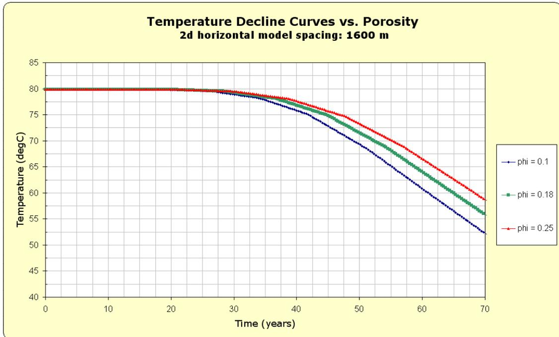
**Figure 13:** Temperature curves for different values for porosity.
