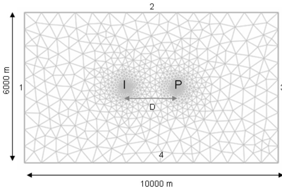
**Figure 8:** Geometry and mesh of the 2d horizontal model
