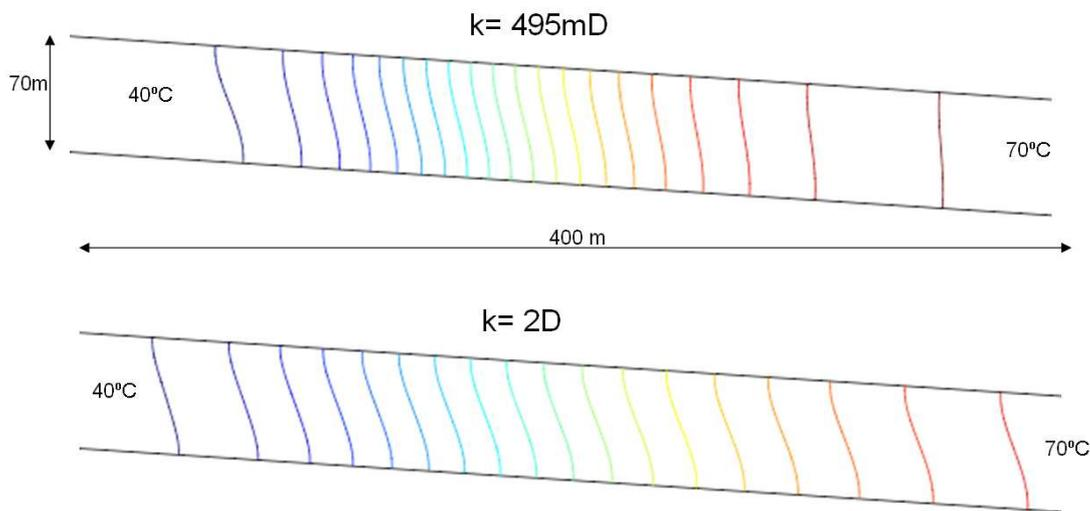
**Figure 6:** Snapshots of the thermal front interval solutions for a permeability of  $k=495\text{mD}$  and  $k=2\text{ D}$ . The coloured lines represent temperature and indirectly viscosity or density.
