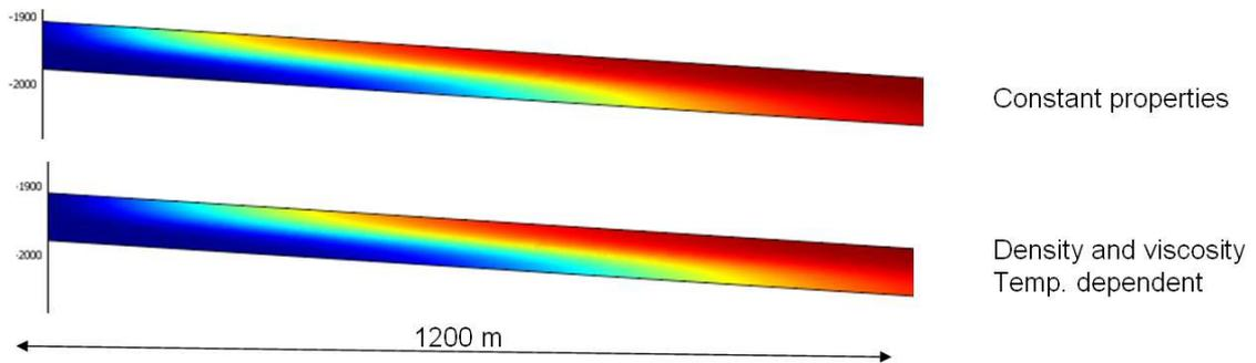
**Figure 7:** Thermal front simulation of cold water injection for a layered system.
