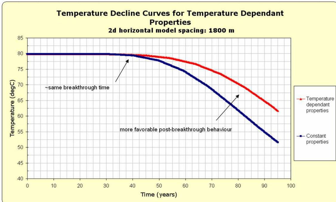
**Figure 14:** Comparison between the use of constant or temperature dependent properties
