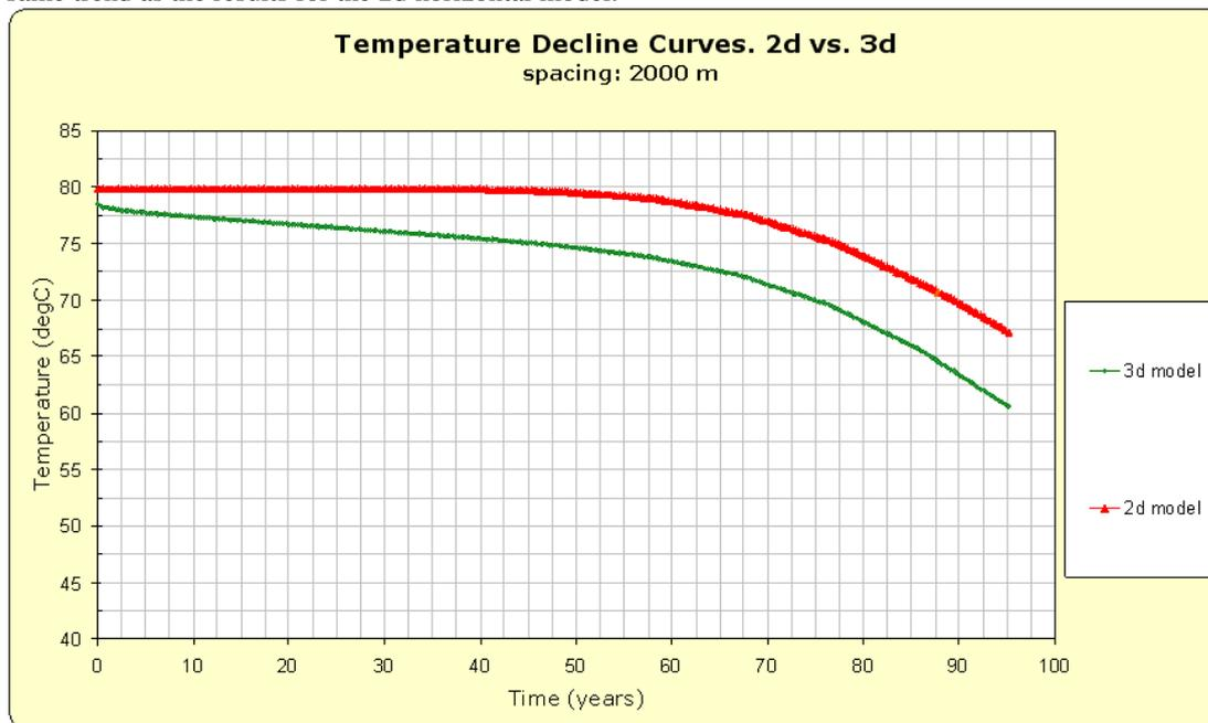
**Figure 16:** Temperature decline curves for 2d horizontal model and 3d model.
