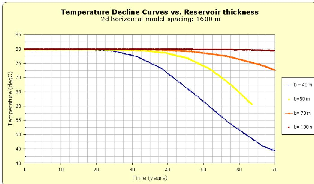
**Figure 12:** Temperature decline curves vs. reservoir thickness for a spacing of 1600 m.
