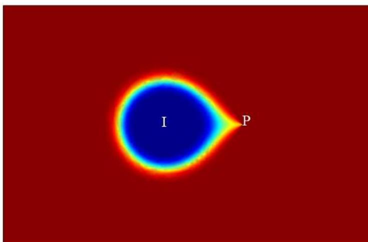
**Figure 9:** Example of typical temperature profile for cold water breakthrough in the 2d horizontal homogeneous model with temperature independent properties.
