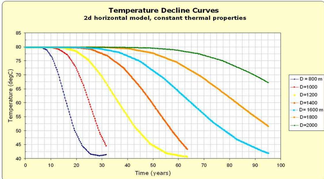
**Figure 10:** Temperature Decline Curves for the 2d horizontal model with temperature independent properties for different values of the inter-well spacing  $D$ .
