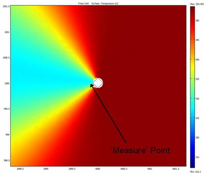
**Figure 11:** ‘Measure’ Point in the model at the production well. The cold water (light blue colour) broke through from the left in this temperature profile.
