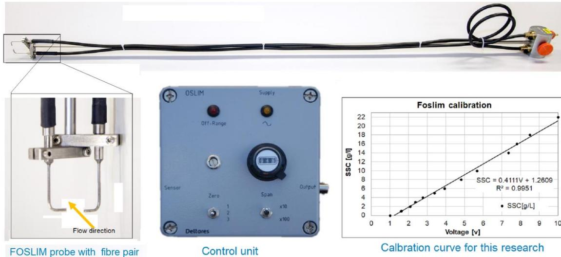
Figure 3-12. FOSLIM components and a calibration curve.
