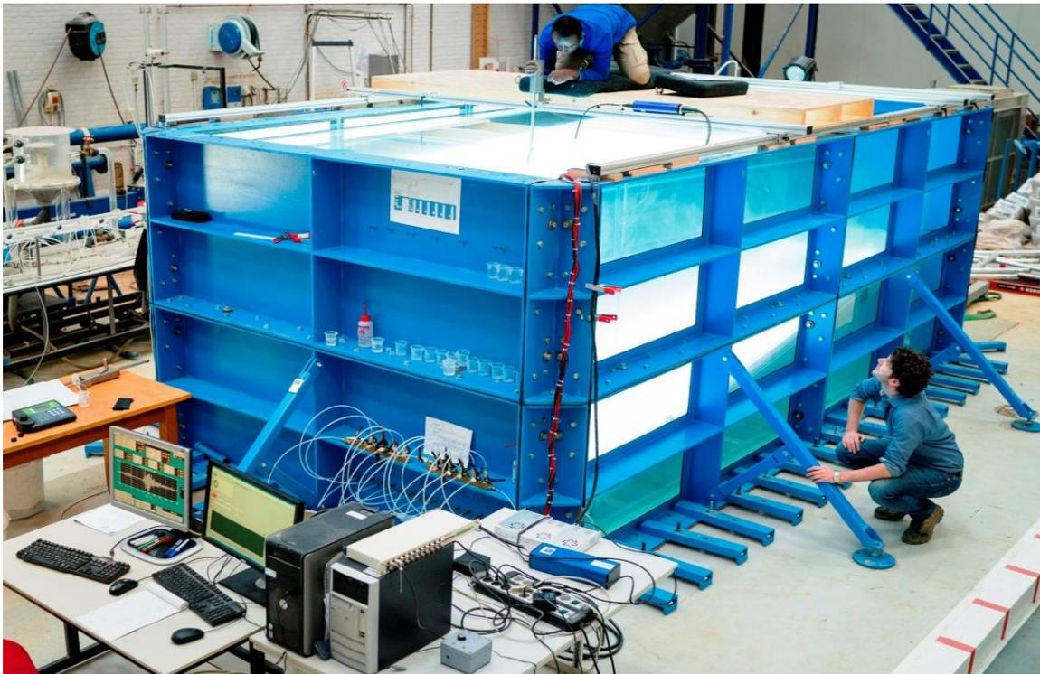
Figure 3-1 Experimental setup. A tank full of 23 m<sup>3</sup> tap water. (Picture was taken by Ivar Pel (© NWO)).
