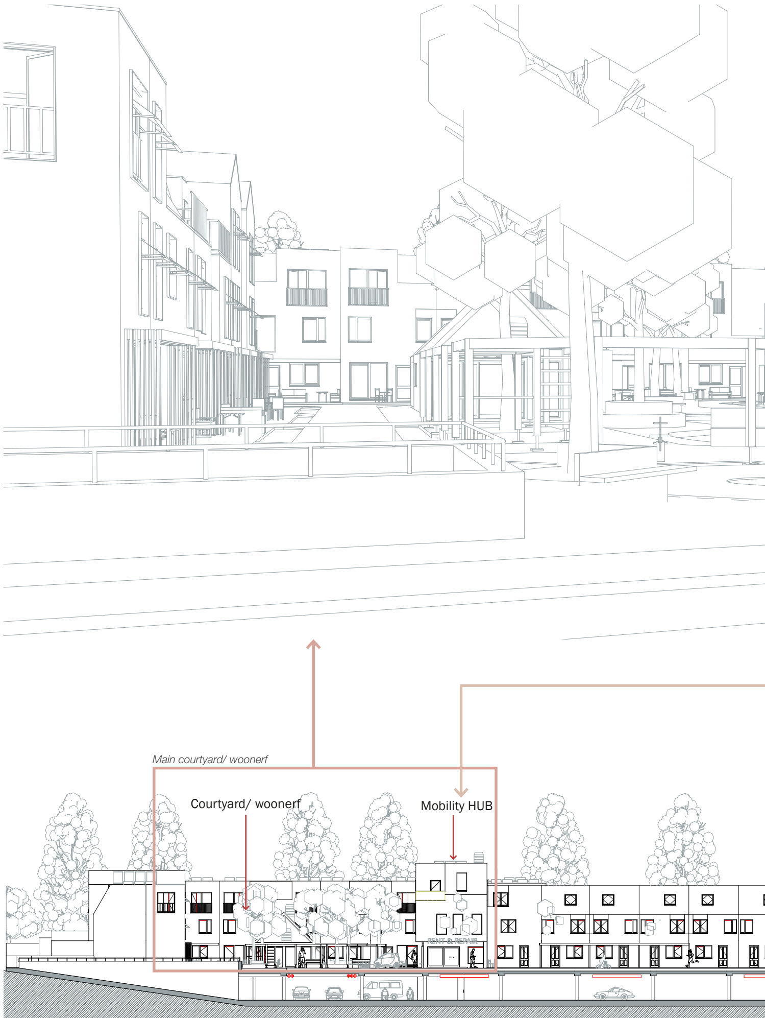
Figure 24: Section G-G, looking from the Dr. J. Presserstraat (main axis) to the courtyards/ woonerven, showing the newly built garage connection
